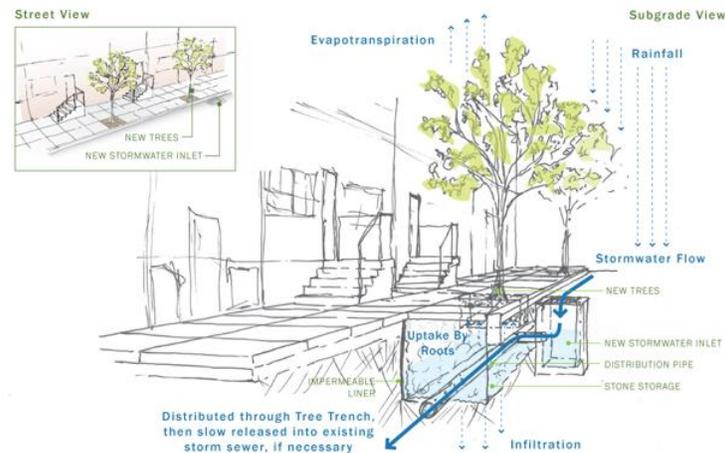
At Right: Graphic rendering of stormwater tree similar to those that will be constructed on this project.
