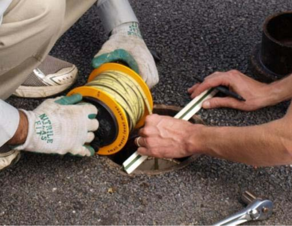
Figure B-1: Manual Water Level Measurement in Observation Well
