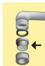
**Aerator Cleaning:** Clean debris from aerators (also called screens) once a month. If aerators are old and worn, replace them with new ones. Aerators should be replaced twice a year.
