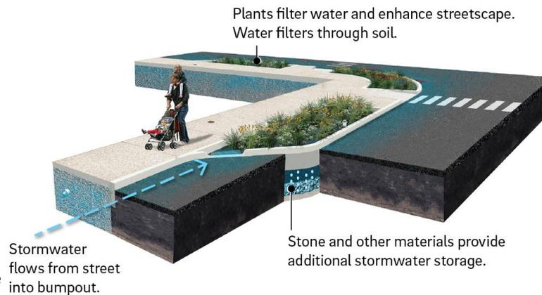
**At Right: Graphic rendering of a completed bumpout similar to the one to be constructed on the northwest corner of Poplar St and N. 40<sup>th</sup> St.**
