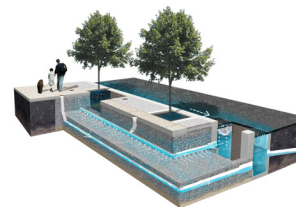
Stormwater Tree Trench
