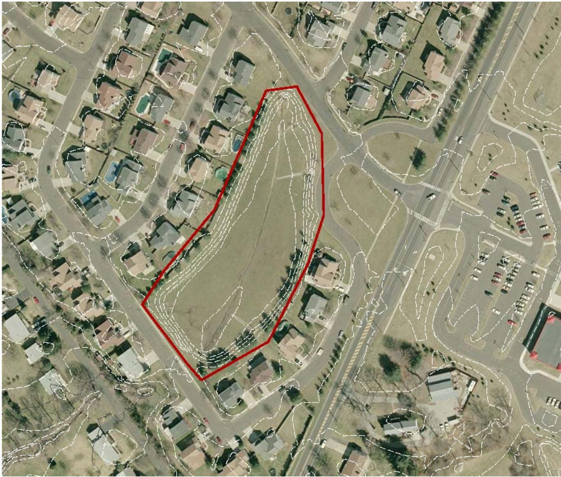
**Figure VI-5 – Typical Stormwater Basin Retrofit**
