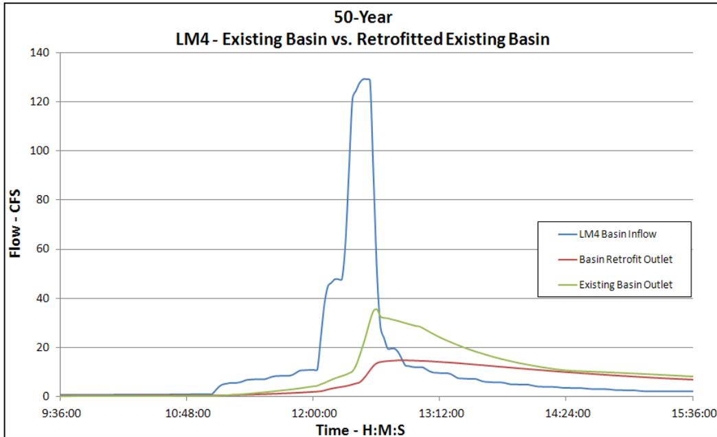
**Figure VI-6: Comparison Hydrograph Outflow from Existing Basin to Retrofitted Basin**
