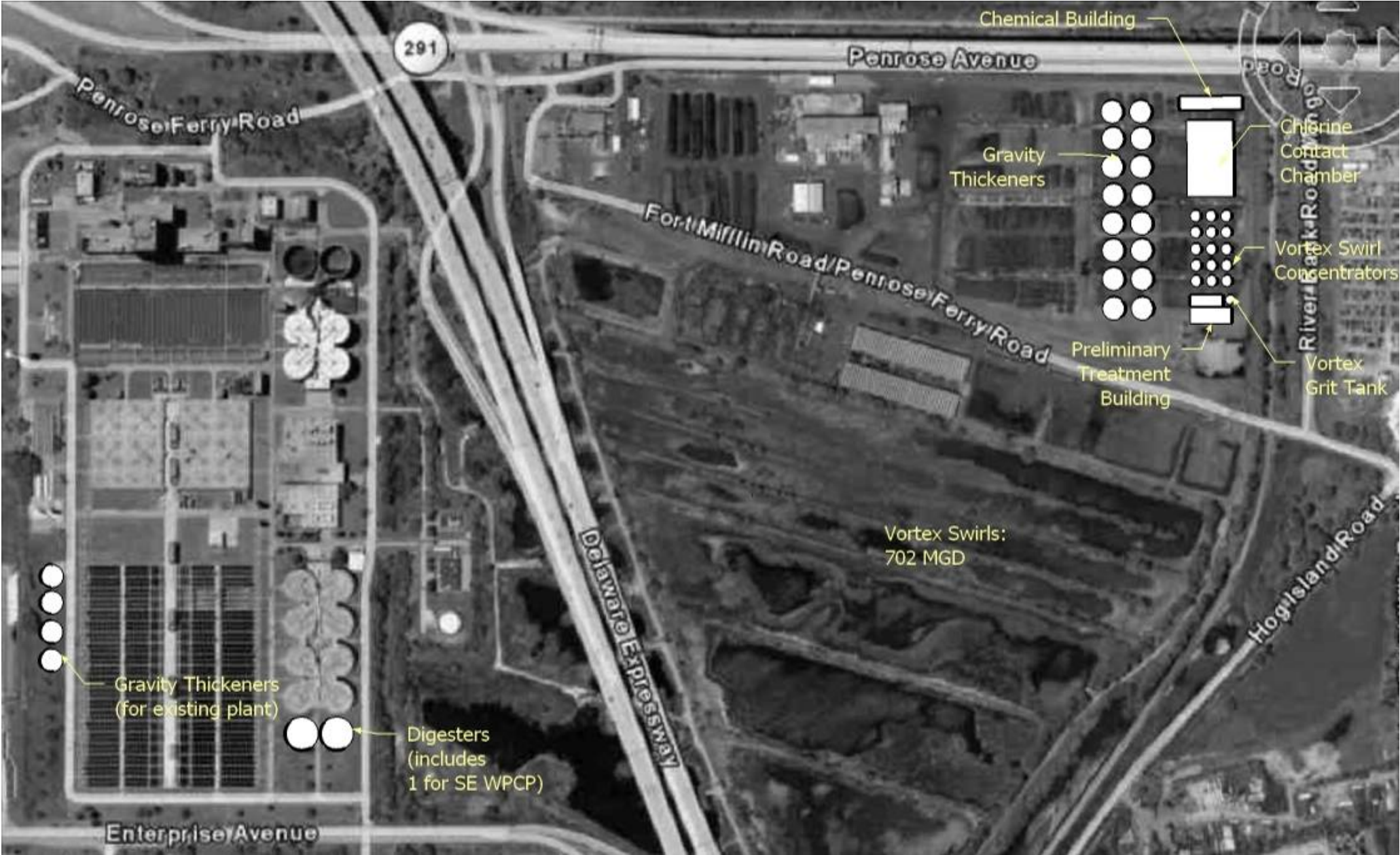
EXHIBIT 5-3 Conceptual Layouts and Footprints for Treatment Train #1: Vortex/Swirl Concentrators 702 MGD Layout
