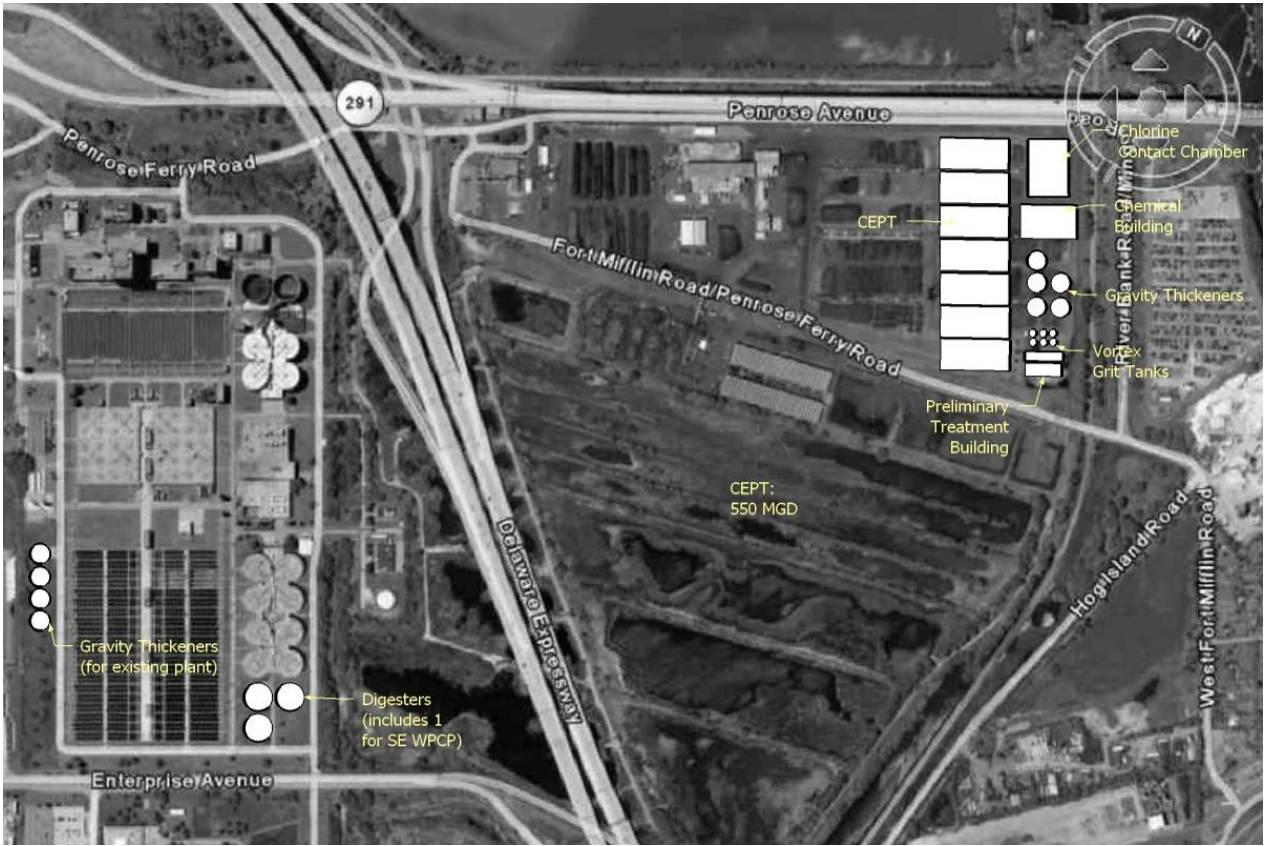
EXHIBIT 7-2 Conceptual Layouts and Footprints for Treatment Train #3: CEPT 550 MGD Layout (left) 1000 MGD (right)
