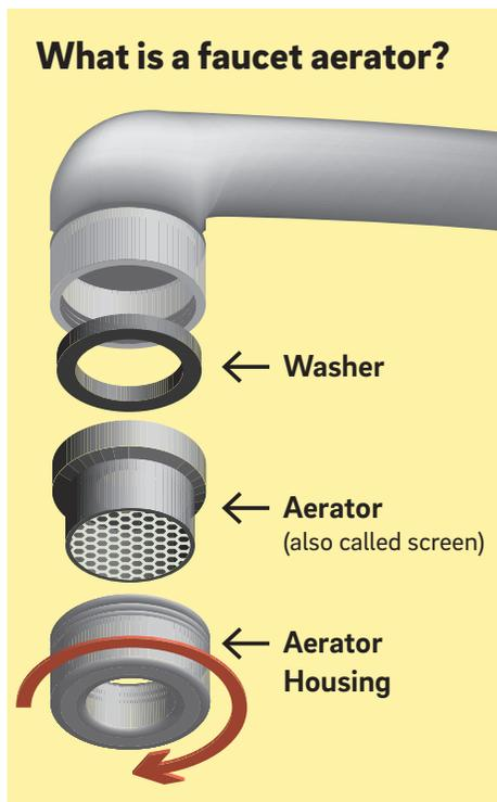
It's a device attached to the tip of a faucet. It saves water, filters out debris, and prevents water from splashing. As water flows through the screen, it mixes with air and flows more evenly.
