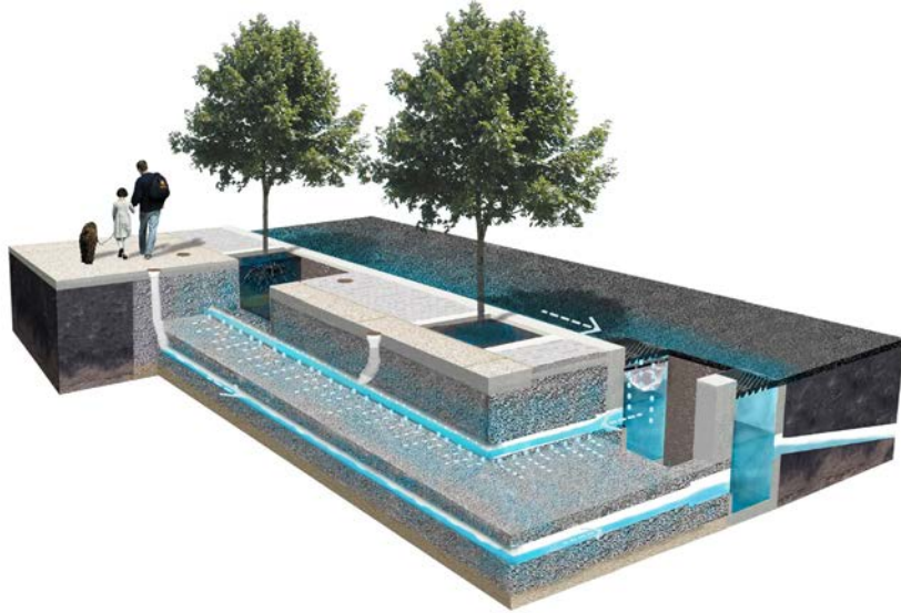
STORMWATER TREE TRENCH
