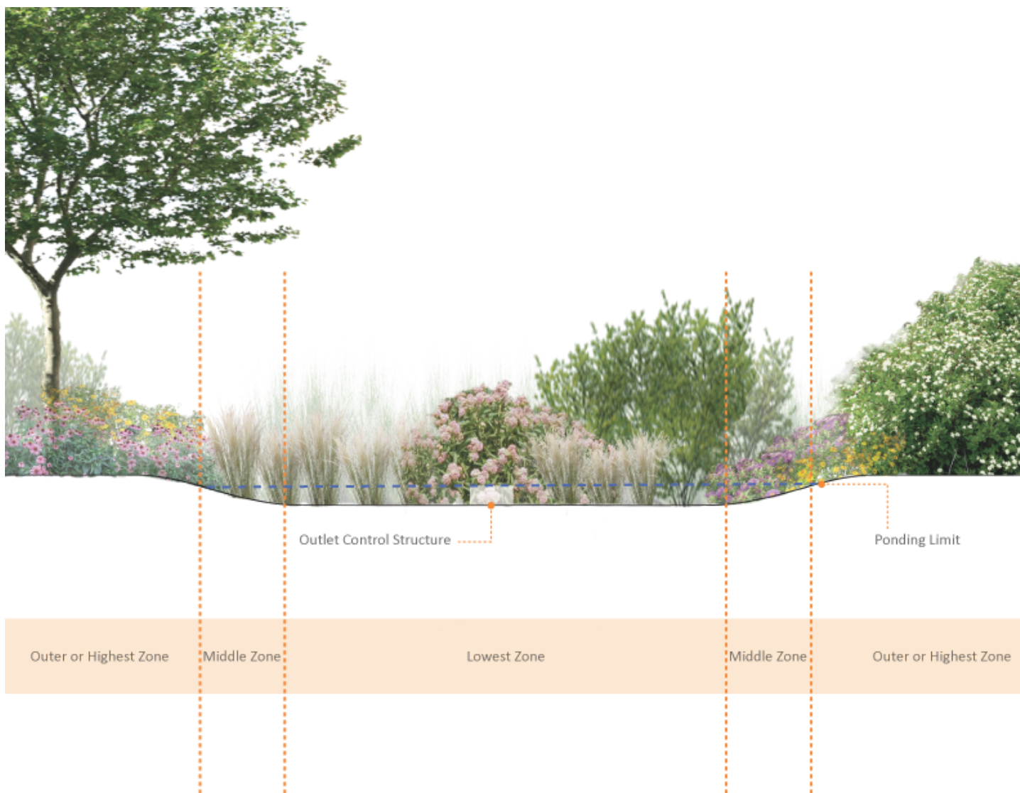
Figure 4.13-3: Hydrologic Zones of a Bioinfiltration/Bioretention Basin
