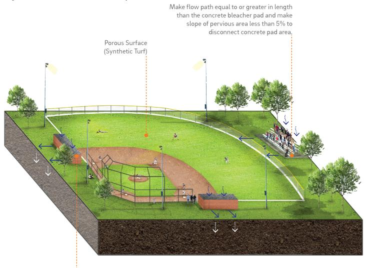
Make flow path equal to or greater in length than the dugout rooftop and make slope of pervious area less than 5% to disconnect roof area.
