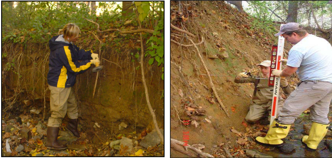
Figure 2-8: Example of bank pin installation (left) and bank pin measurement (right) by PWD staff
