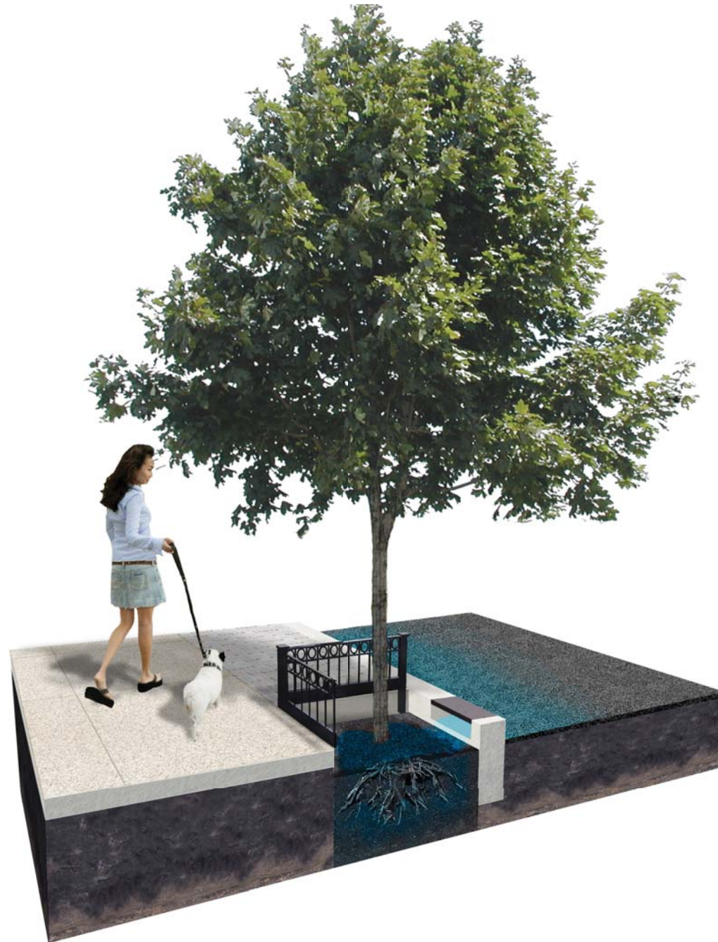
Figure 1-19. Stormwater Tree with Typical Features
