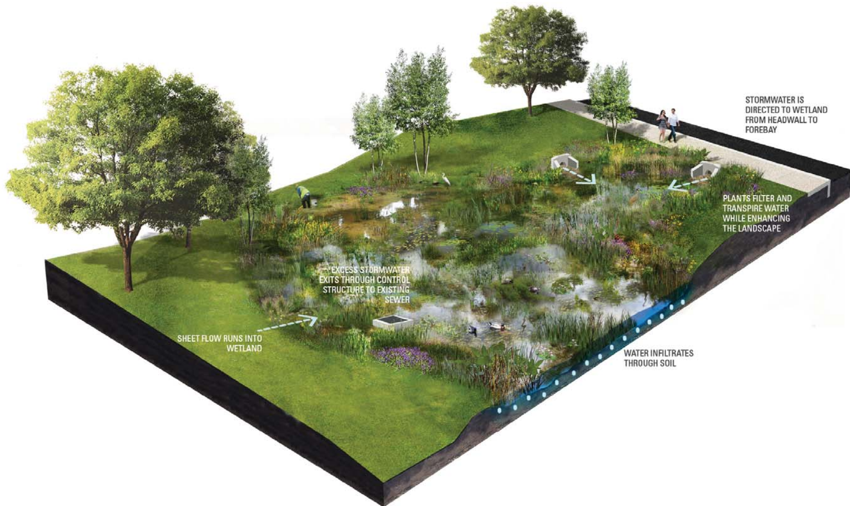
Figure 1-13. Stormwater Wetland with Typical Features
