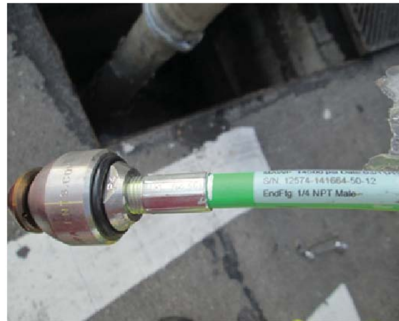
Figure 3-7: Small rotating, root cutting nozzle
