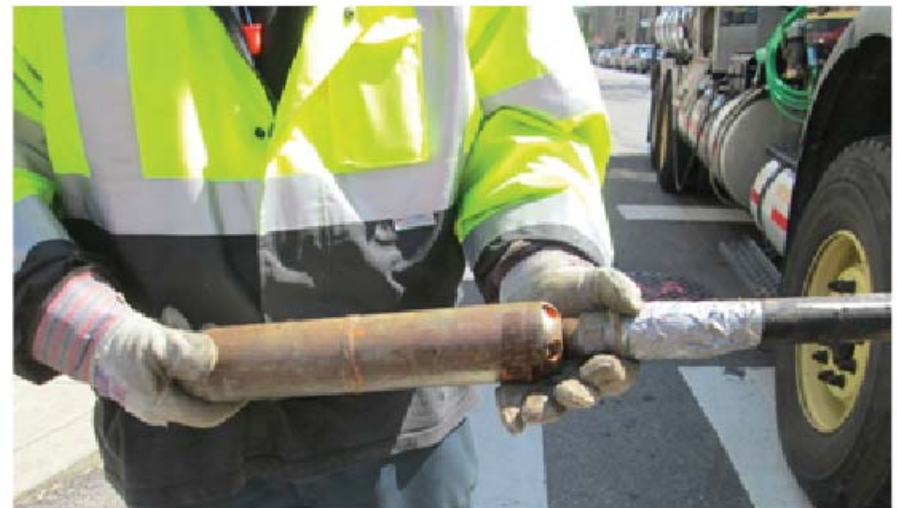
Figure 3-4. Large penetrating nozzle with one front-facing and five-rear facing jets
