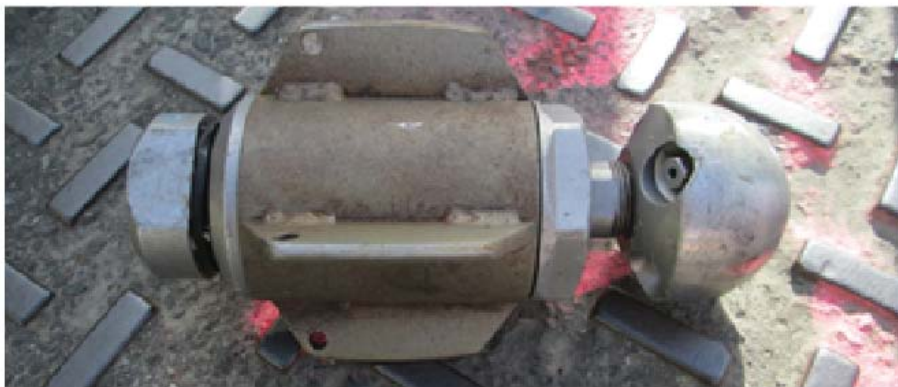
Figure 3-6. Rotating nozzle with three rear-facing jets and rotating center
