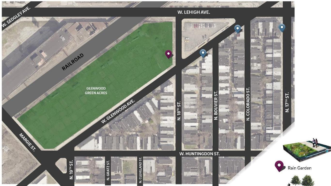
These GSI systems capture and store stormwater runoff to protect local waterways. Concept subject to change.
