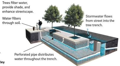
At Right: Graphic rendering of the Tree Trench similar to the one to be installed at W. Sedgley Avenue near N. 19th Street.
