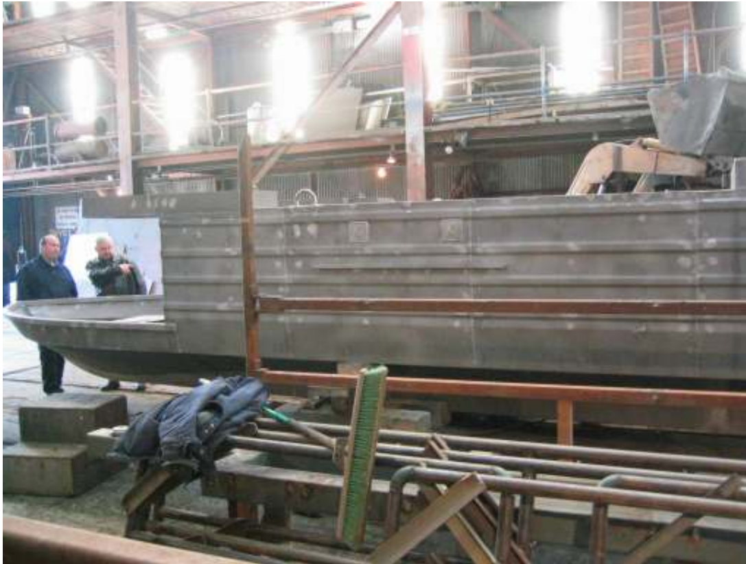
Figure 1. Completion of Bare-Hull Component of Skimming Vessel as seen during December Inspection.
