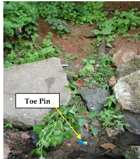
Figure 9 - Bank Pin Monitoring Site showing installation of toe pin relative to bank pin locations
