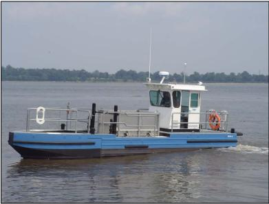
Figure II.F-3 Floatables Skimming Vessel in operation
