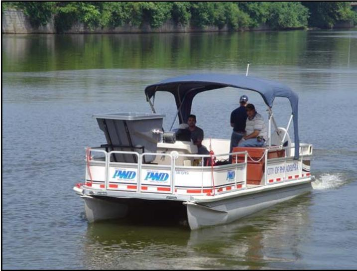
**Figure II.F-4 Floatables Pontoon Vessel in operation**
