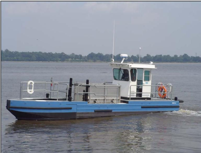
**Figure II.F-3 Floatables Skimming Vessel in operation**
