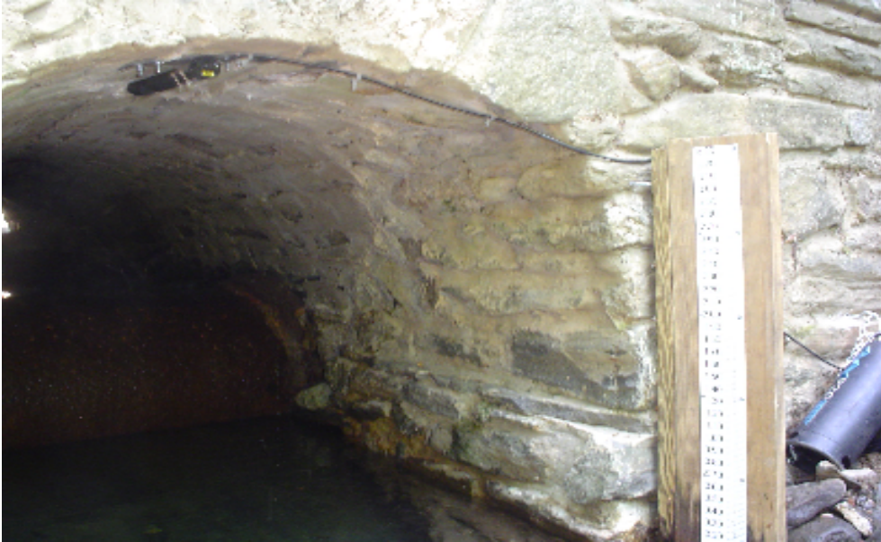
Appendix C, Figure 10 - An ultrasonic down-looking acoustic water level sensor for water level measurement as it was installed above the Cathedral Run tributary
