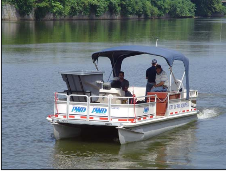
Figure II.F-4 Floatables Pontoon Vessel in operation
