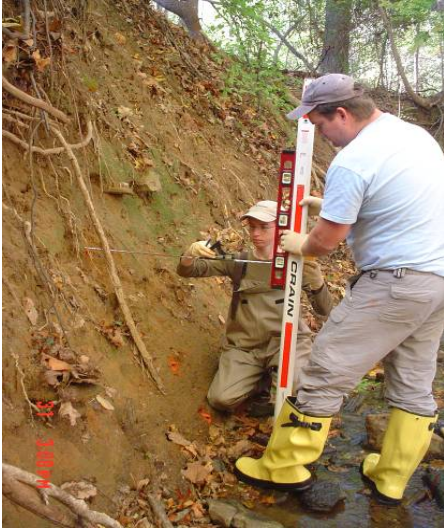
Figure 2.4.4: The survey rod measures the amount of exposed pin and the amount of lateral erosion upon re-survey
