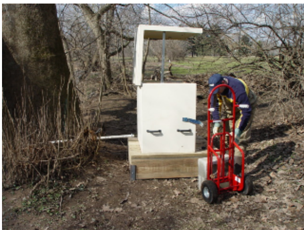
Appendix C, Figure 9 - PWD staff setting up the automated water sampler for wet weather monitoring
