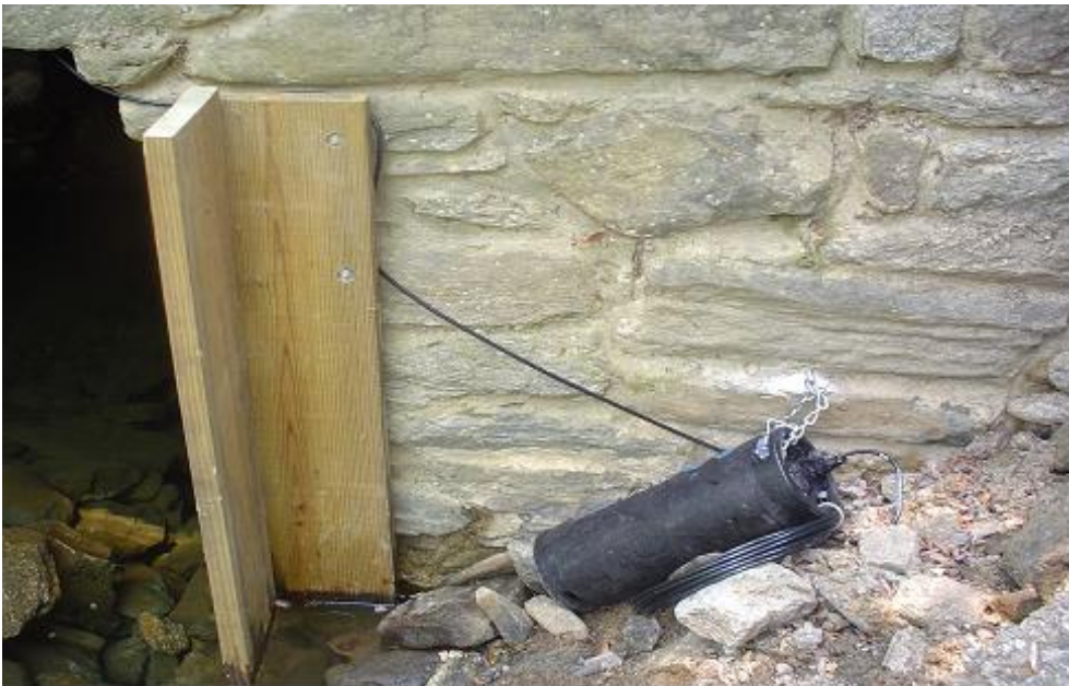
Appendix C, Figure 11 - A pressure transducer for redundant water level measurement as it was installed in the Cathedral Run tributary.
