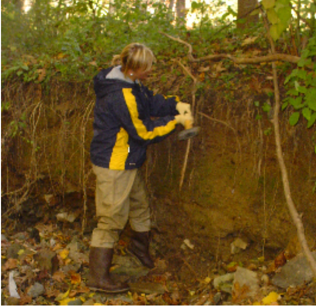
Appendix C, Figure 2 - PWD staff installing a bank pin into the bank along the Wisers Mill tributary. Bank pins are driven horizontally into streambanks at positions corresponding to bank erosion locations.
