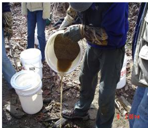
Appendix C, Figure 7 - PWD staff collected a bar sample representing the size gradation of bedload at the bankfull stage.
