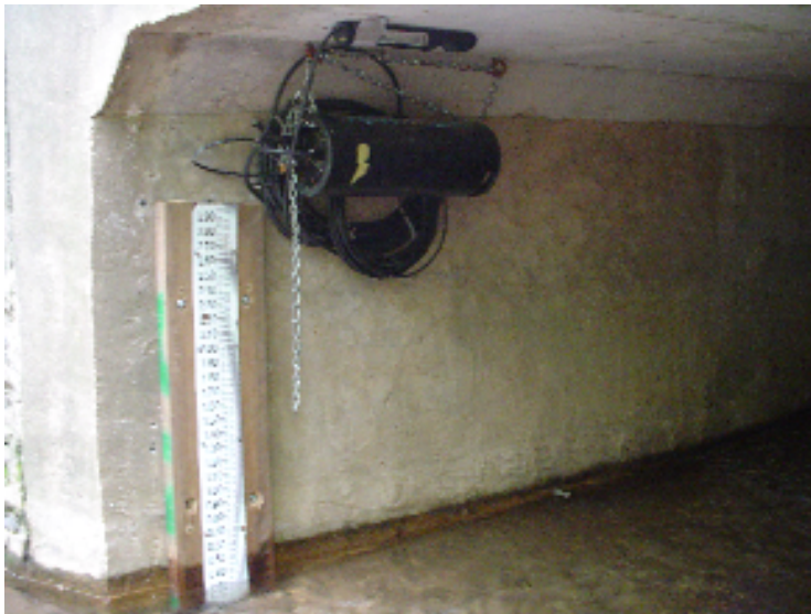
Appendix C, Figure 13 - Staff Gage for the Bells Mill tributary pictured with a pressure transducer and ultrasonic down-looking sensor.
