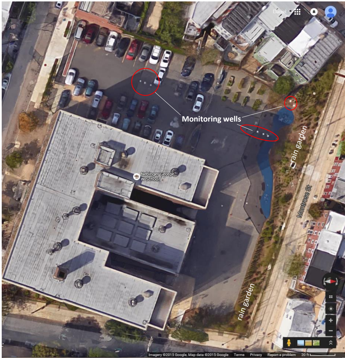
Figure 8 Recent aerial photograph showing the rain garden and surrounding wells at George W. Nebinger School (from Google, 2015).
