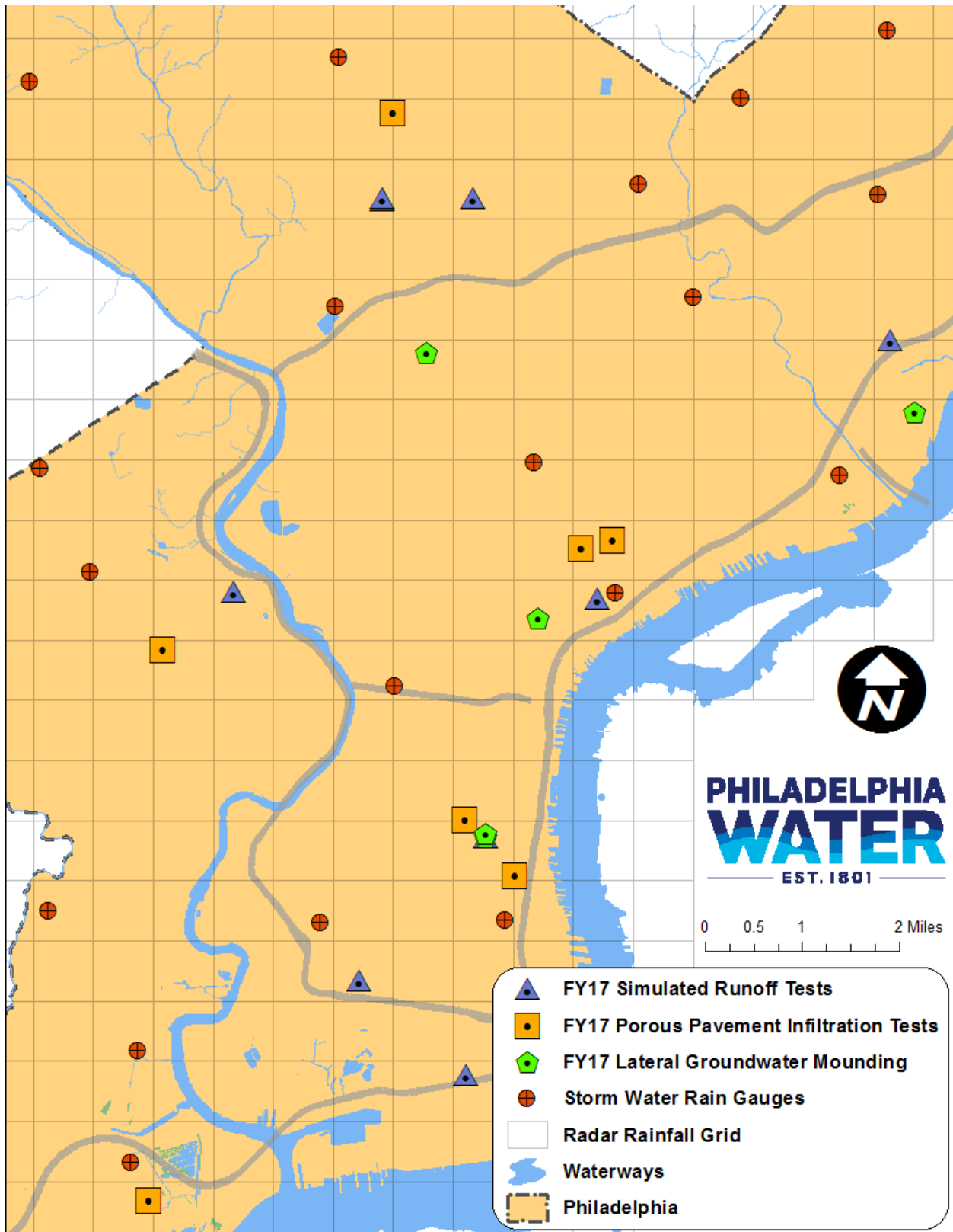
Figure 3-2: Lateral Groundwater Mounding Monitoring, Simulated Runoff Testing and Surface Infiltration Testing Locations
