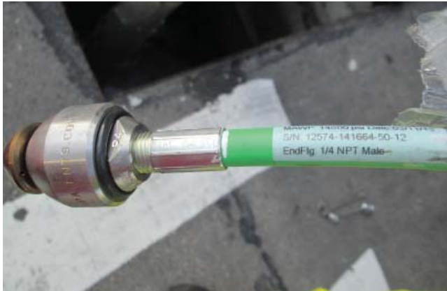
Figure 3-6: Small Rotating, Root Cutting Nozzle
