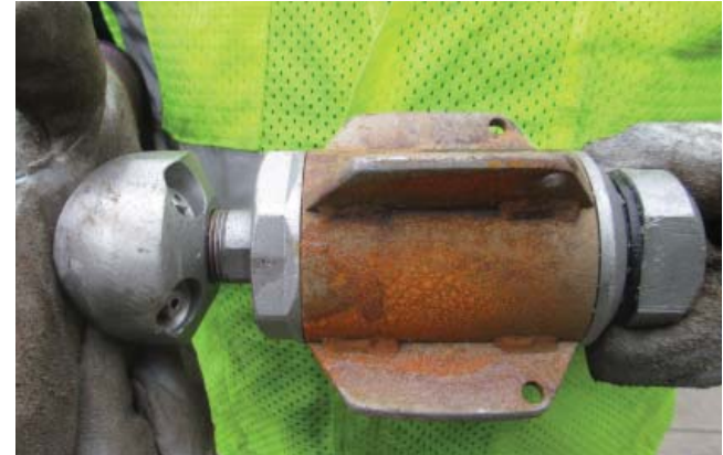
Figure 3-5. Most Commonly Used Nozzle. Rotating Nozzle with 3 Rear-facing Jets and Rotating Center
