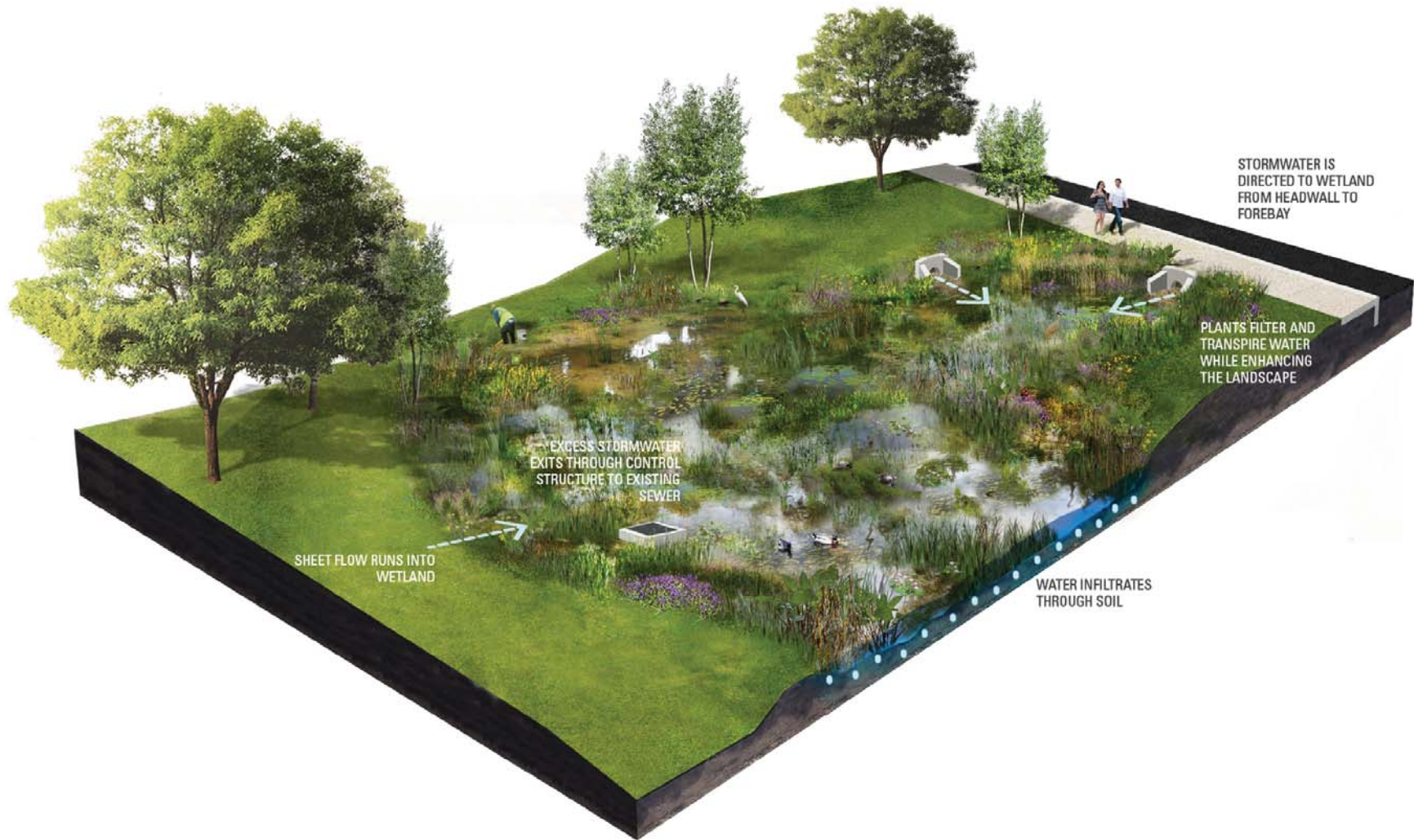
Figure 1-16. Stormwater Wetland with Typical Features
