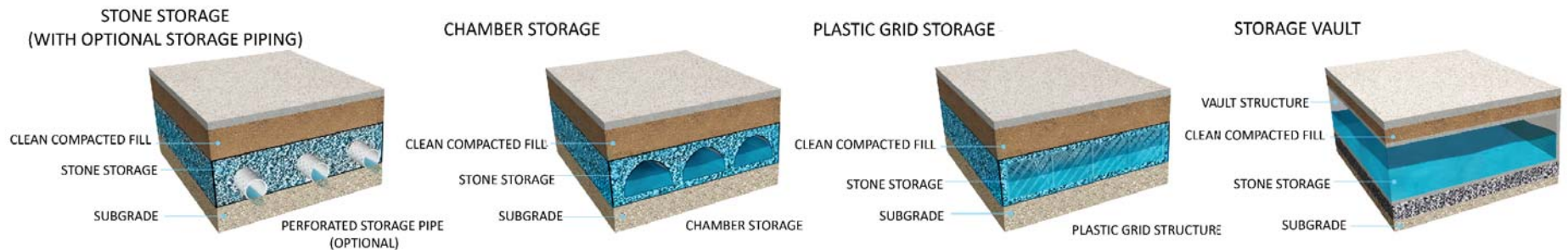
Figure 1-14. Infiltration/Storage Trench with Typical Features
