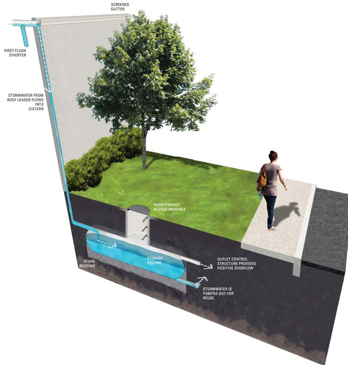
Figure 1-28. Subsurface Cistern with Typical Features
