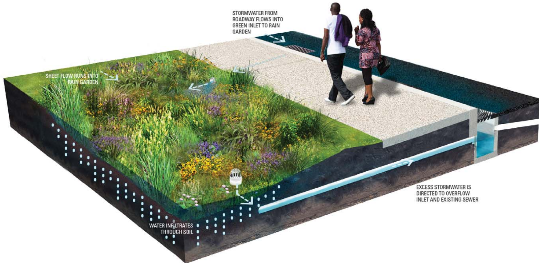
Figure 1-4. Rain Garden with Typical Features
