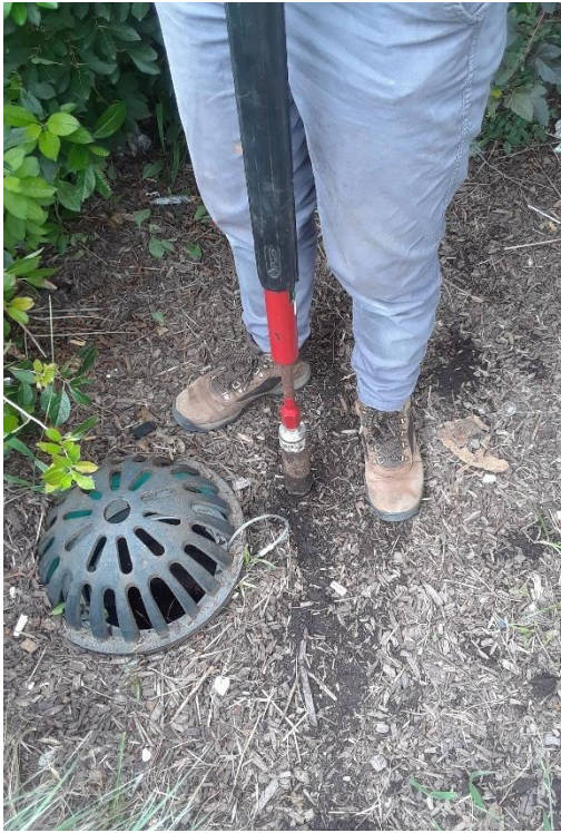
Figure 5-7 – Using soil core sampler (left) to dig shallow well hole (right)
