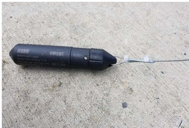
Figure 5-3 – Sensor and stainless-steel cable attachment
