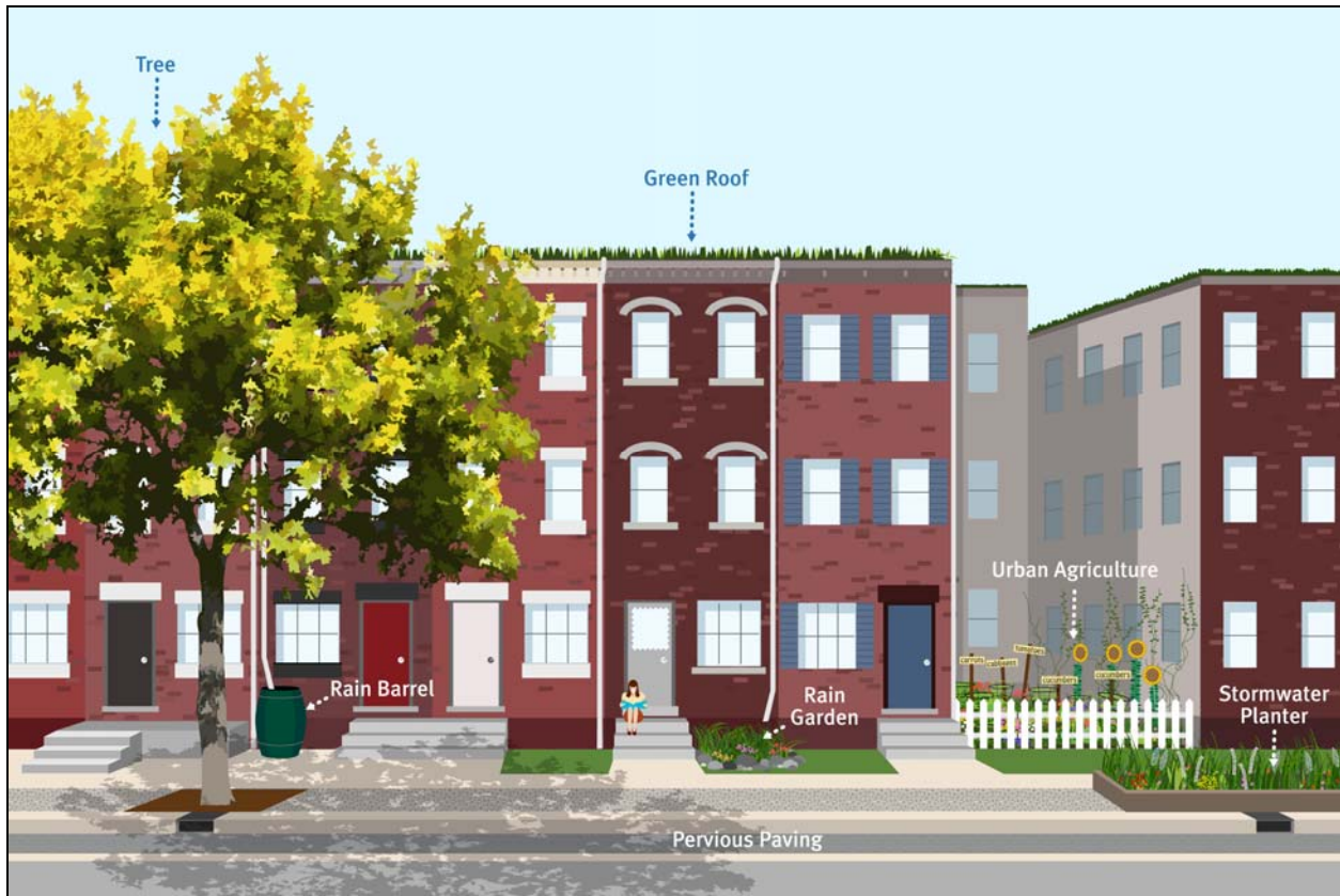
Figure 10-5 Graphic of a City Neighborhood with Green Stormwater Infrastructure Components Implemented (Source: WRT Designs)
