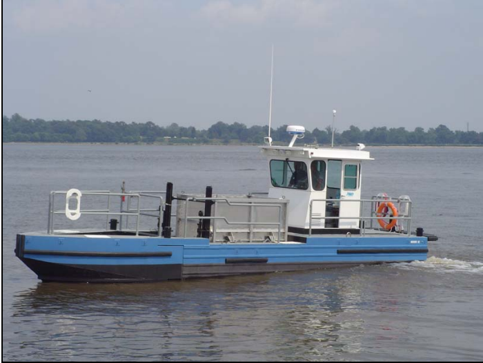
Figure 10-32 Floatables Skimming Vessel in Operation
