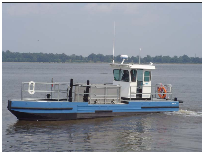
Figure 10-32 Floatables Skimming Vessel in Operation
