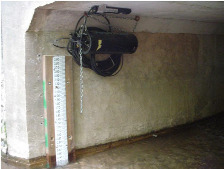
**Appendix A, Figure 13 - Staff Gage for the Bells Mill tributary pictured with a pressure transducer and ultrasonic down-looking sensor.**
