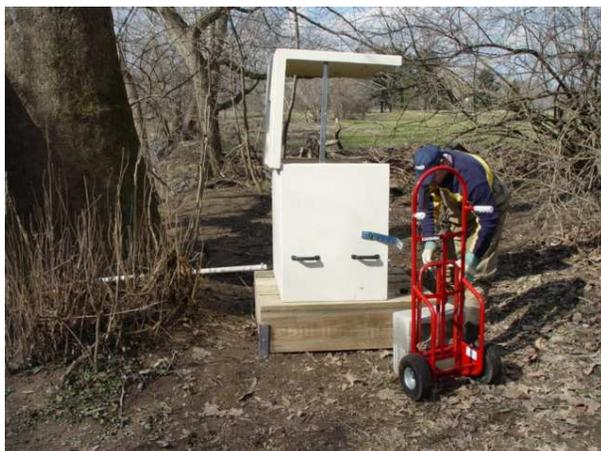
**Appendix A, Figure 9 - PWD staff setting up the automated water sampler for wet weather monitoring**
