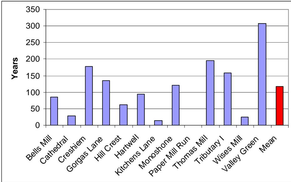
Appendix A, Figure 16 - Estimated erosion rate based on BEHI/NBS from current cross section data.
