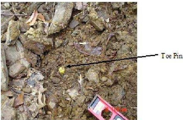
**Appendix A, Figure 6 - The toe pin is a permanent reference point for determining lateral erosion.**
