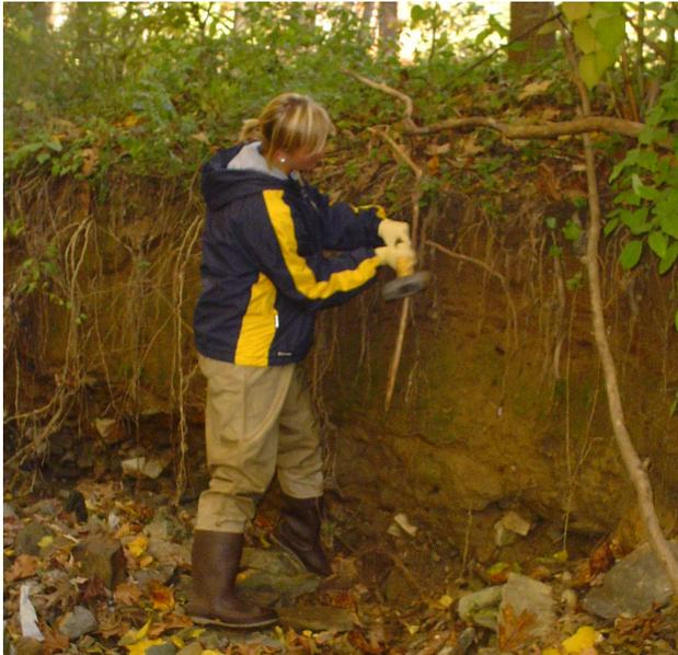
**Appendix A, Figure 2 - PWD staff installing a bank pin into the bank along the Wises Mill tributary. Bank pins are driven horizontally into streambanks at positions corresponding to bank erosion locations.**
