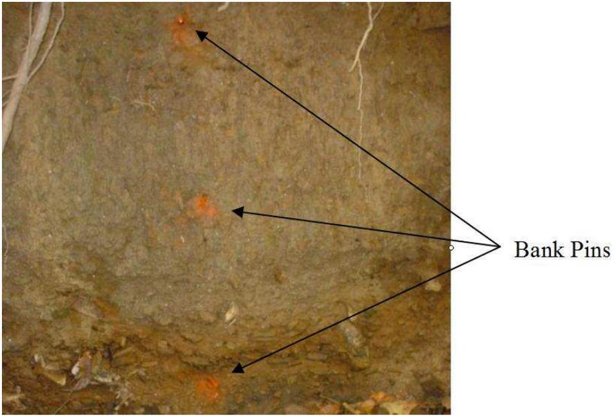
**Appendix A, Figure 3 - After bank pin installation, the exposed ends were spray painted to make more visible**
