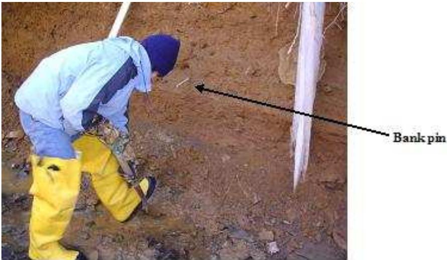
**Appendix A, Figure 1 - PWD staff digging out eroded bank sediment in order to accurately measure bank pin exposure**
