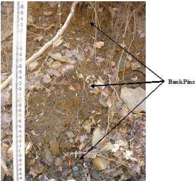
**Appendix A, Figure 5 - The survey rod measures the amount of exposed pin as the amount of lateral erosion upon re-survey.**
