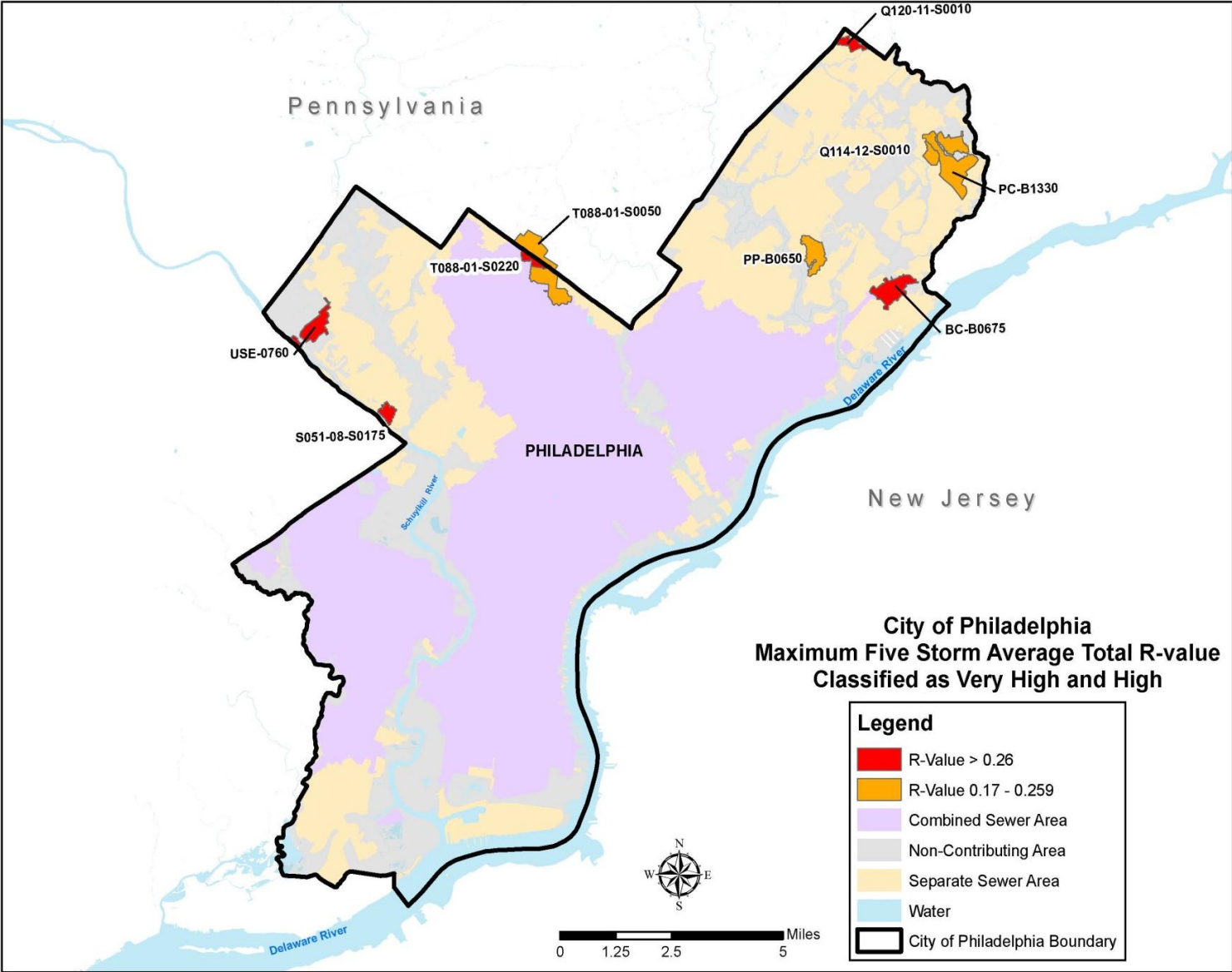
Figure 4-19: Identified Sanitary Sewershed Areas with the Highest RDII Flow – Maximum Five Storm Average Total R-Value Analysis Method
