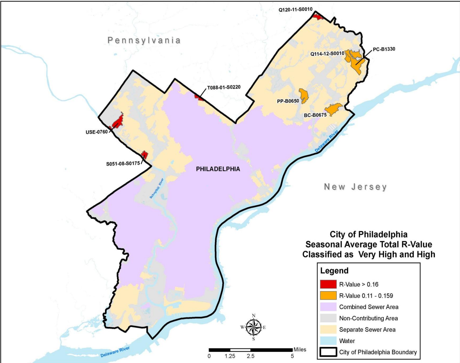
Figure 4-20: Identified Sanitary Sewershed Areas with the Highest RDII Flow – Maximum Seasonal Average Total R-Value Analysis Method
