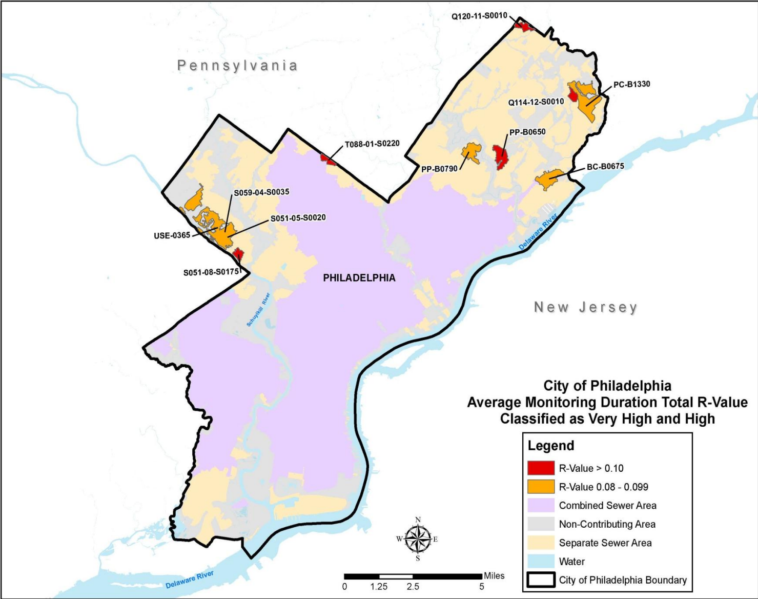
Figure 4-21: Identified Sewershed Areas with the Highest RDII Flow – Average Monitoring Duration Total R-Value Analysis Method
