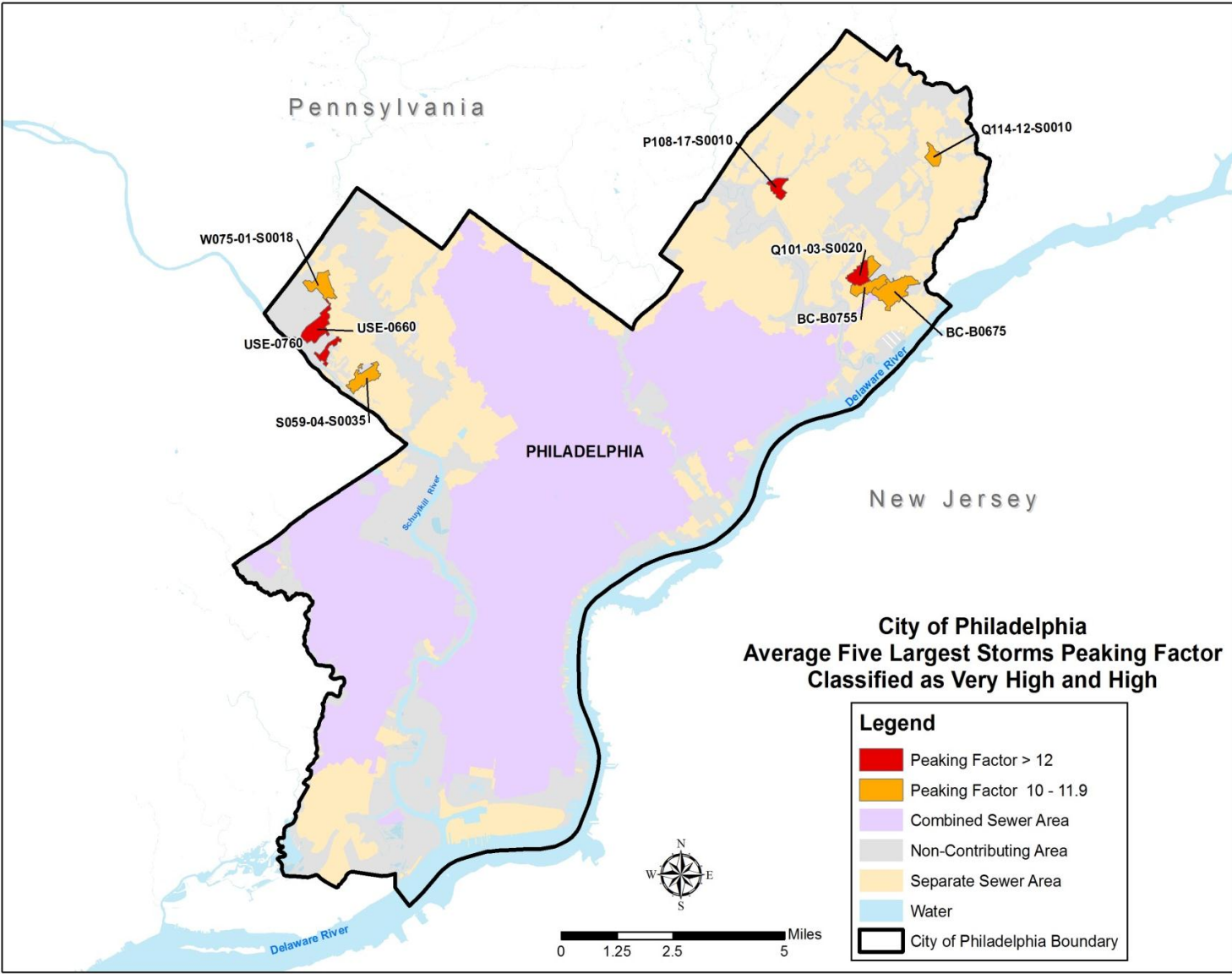
Figure 4-22: Identified Sewershed Areas with the Highest RDII Flow – Site Average Five Largest Storm Peaking Factor Analysis Method
