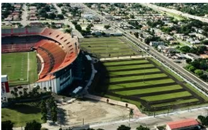
A green parking lot at the Orange Bowl in Miami, Florida (Source: Invisible Structures, no date)
