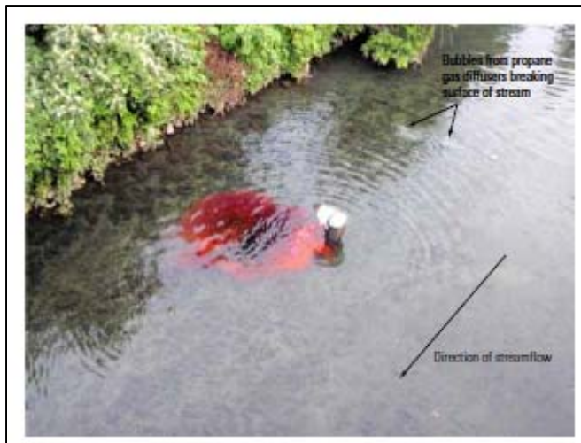
Figure 3-10: Dye Injection and Propane Gas Diffusion on September 3, 2009 in TTF Creek near US Route 1 (from Senior and Gyves, 2010)
