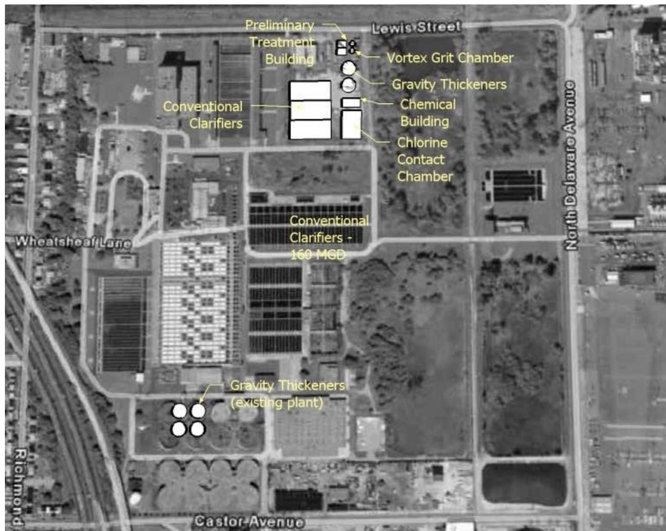
EXHIBIT 5-2 Conceptual Layouts and Footprints for Treatment Train #2: Conventional Clarifiers 160 MGD 160 MGD (left), 376 MGD (right)
