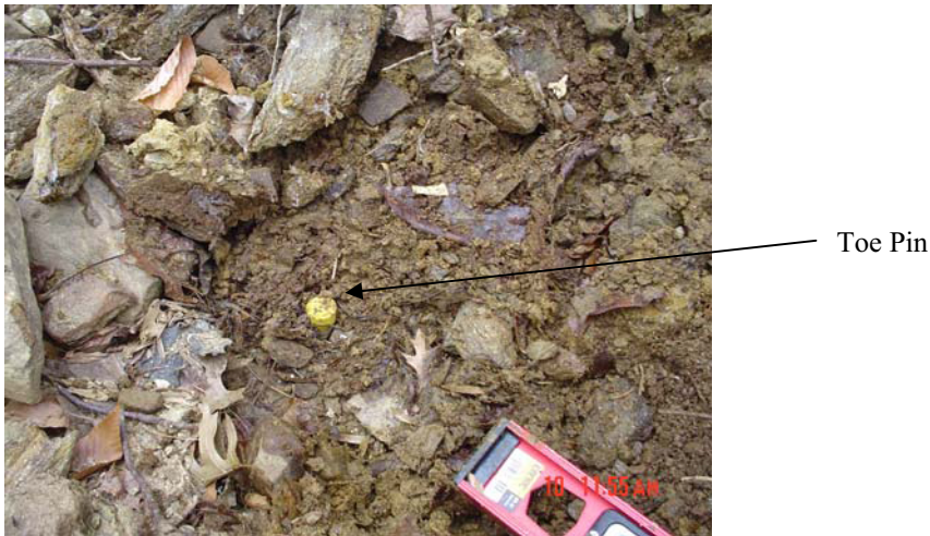
Figure J-4 Toe Pin Installed in a Wissahickon Tributary
