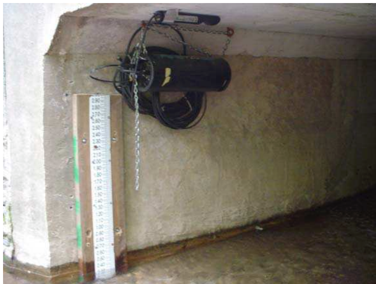
Figure J-10 Staff Gage, Pressure Transducer, and Ultrasonic Down-looking Sensor in Bells Mill Tributary
