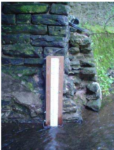
Figure J-9 Pressure Transducer for Water Level Measurement Installed in Monoshone Tributary
