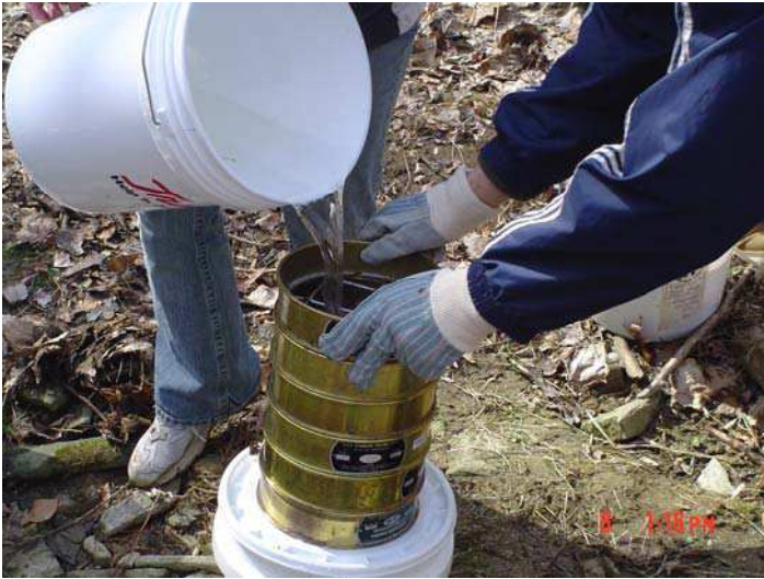
Figure J-6 Sieving During Bar Sample Collection
