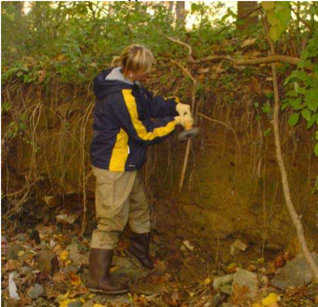
Figure J-2 Bank Pin Installation in Wises Mill Tributary
