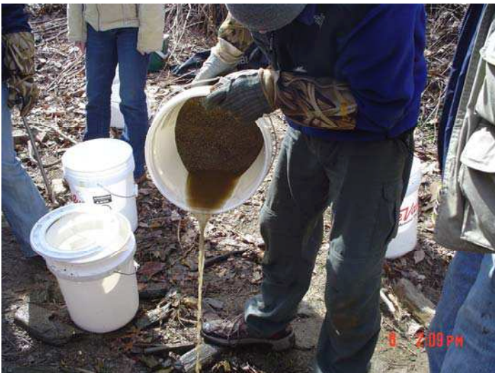
Figure J-7 Draining Water During Bar Sample Collection
