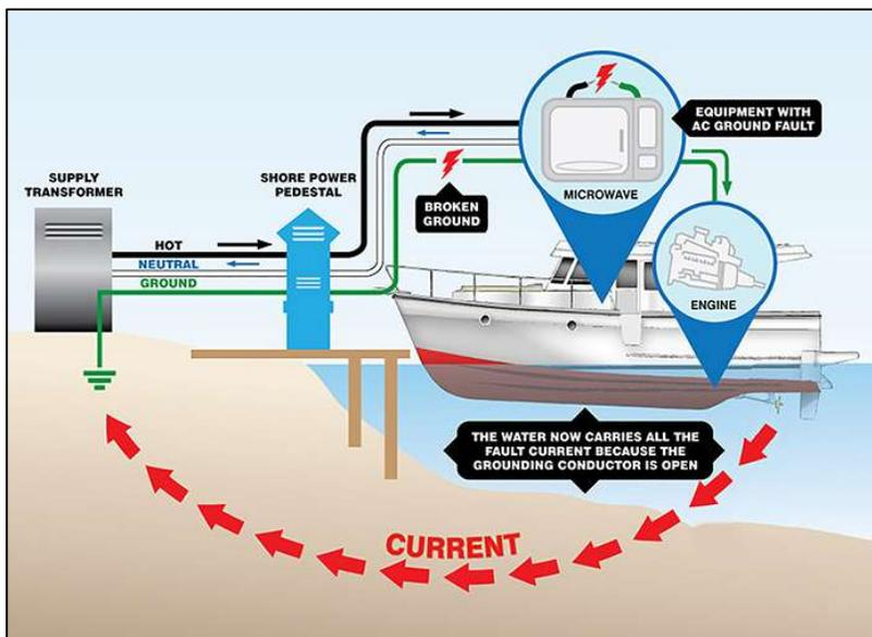
**Figure 6.7 How Electrical Current can Leak into the Water (Boat U.S.)**
