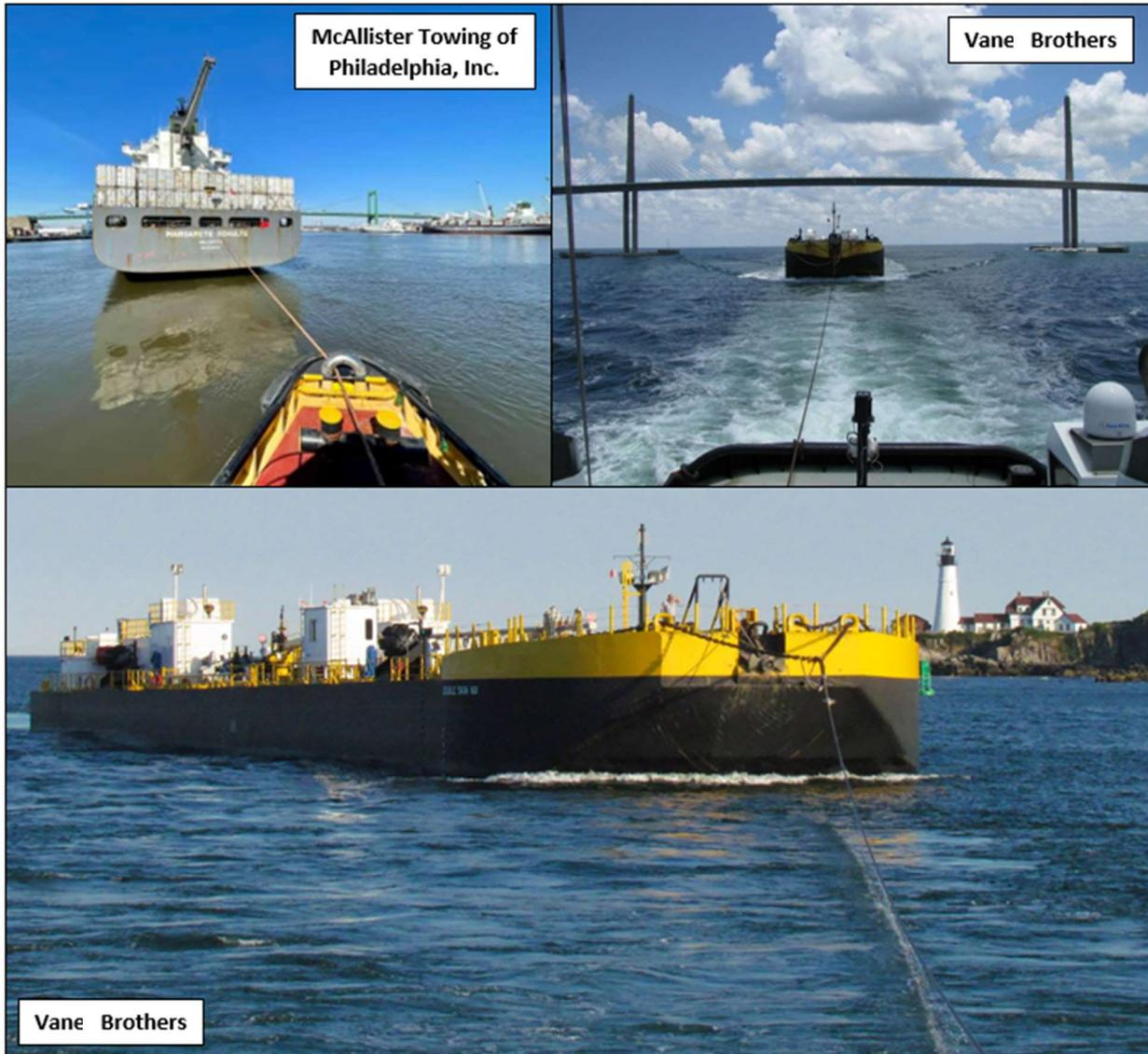
**Figure 7.4 Towlines Located Above the Water Surface**
