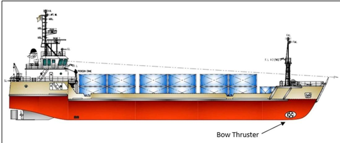
**Figure 7.2 Diagram Showing a Bow Thruster on a Container Ship (Baird Maritime)**
