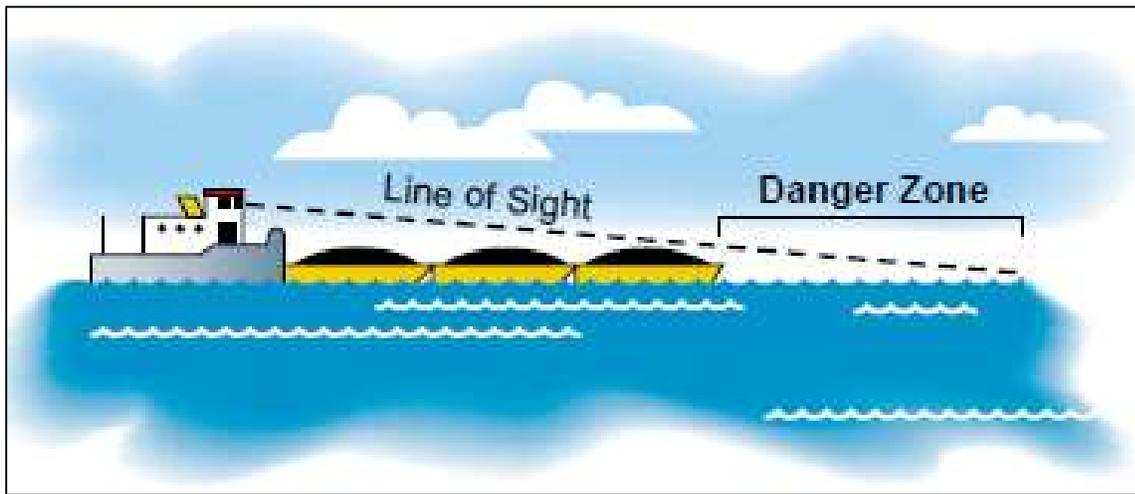
**Figure 7.13 Tugboat Blind Spot Extends Hundreds of Feet (American Waterways Operators)**
