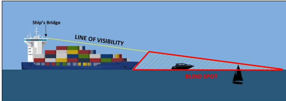
**Figure 7.11 Blind Spot Ahead of the Bow Extends Hundreds of Feet (The Chart Room)**
