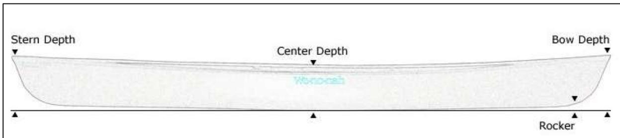
**Figure 8.18 Center Depth Measurement in Canoes (Wenonah Canoe)**
