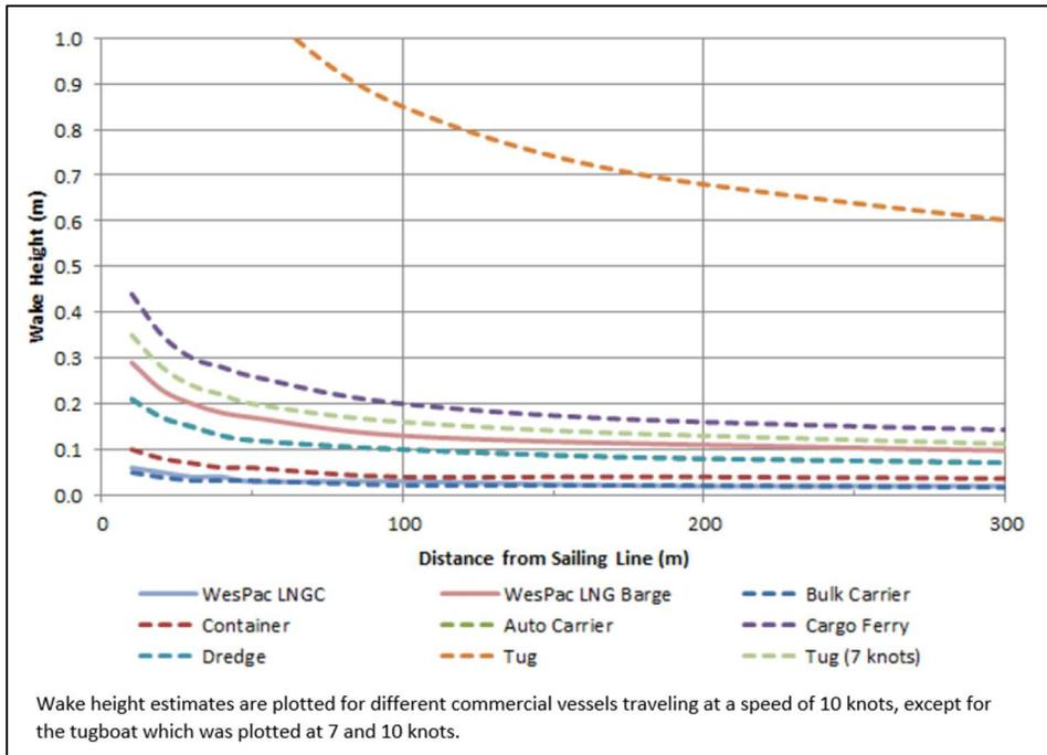
**Figure 7.19 Wake Heights for Commercial Vessels (Ausenco Engineering Canada Inc., 2015)**
