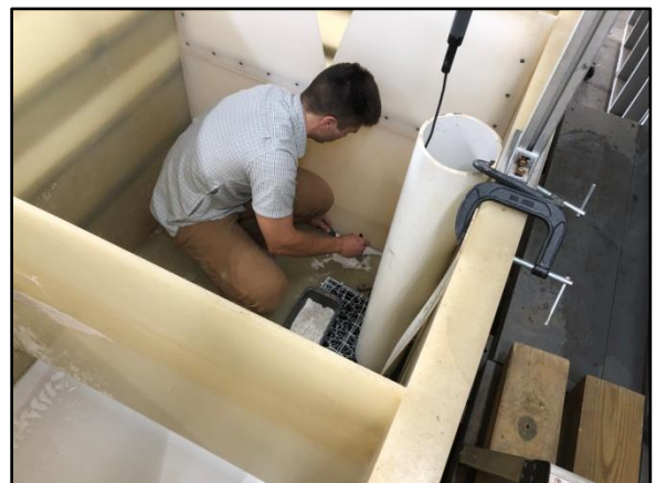
Figure 4. SCC Mass Loading Capacity – Monitoring Head and Collecting Passing Sediments
