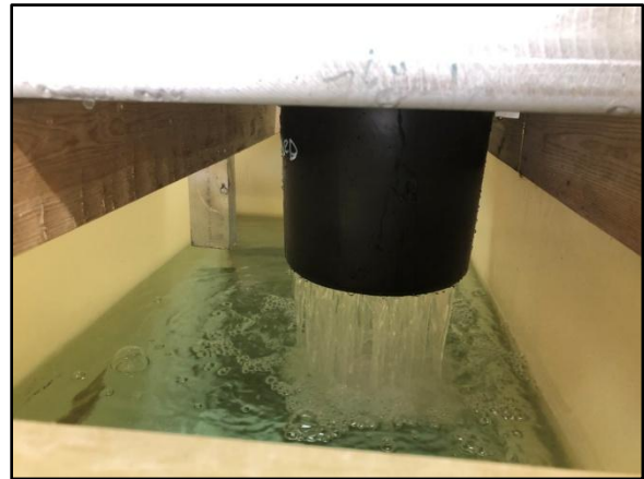
Figure 3. SCC Removal Efficiency – Sediment Augered into Flow; Influent & Effluent Sampled
