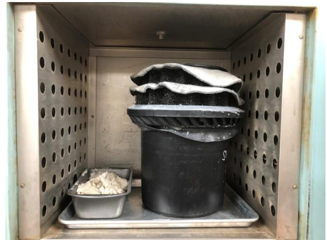
Drying of Sediment-laden Cartridge and Collected Retained Sediments (typical)
