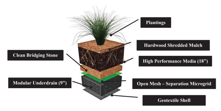
Figure 1 FocalPoint HPMBS System Components
