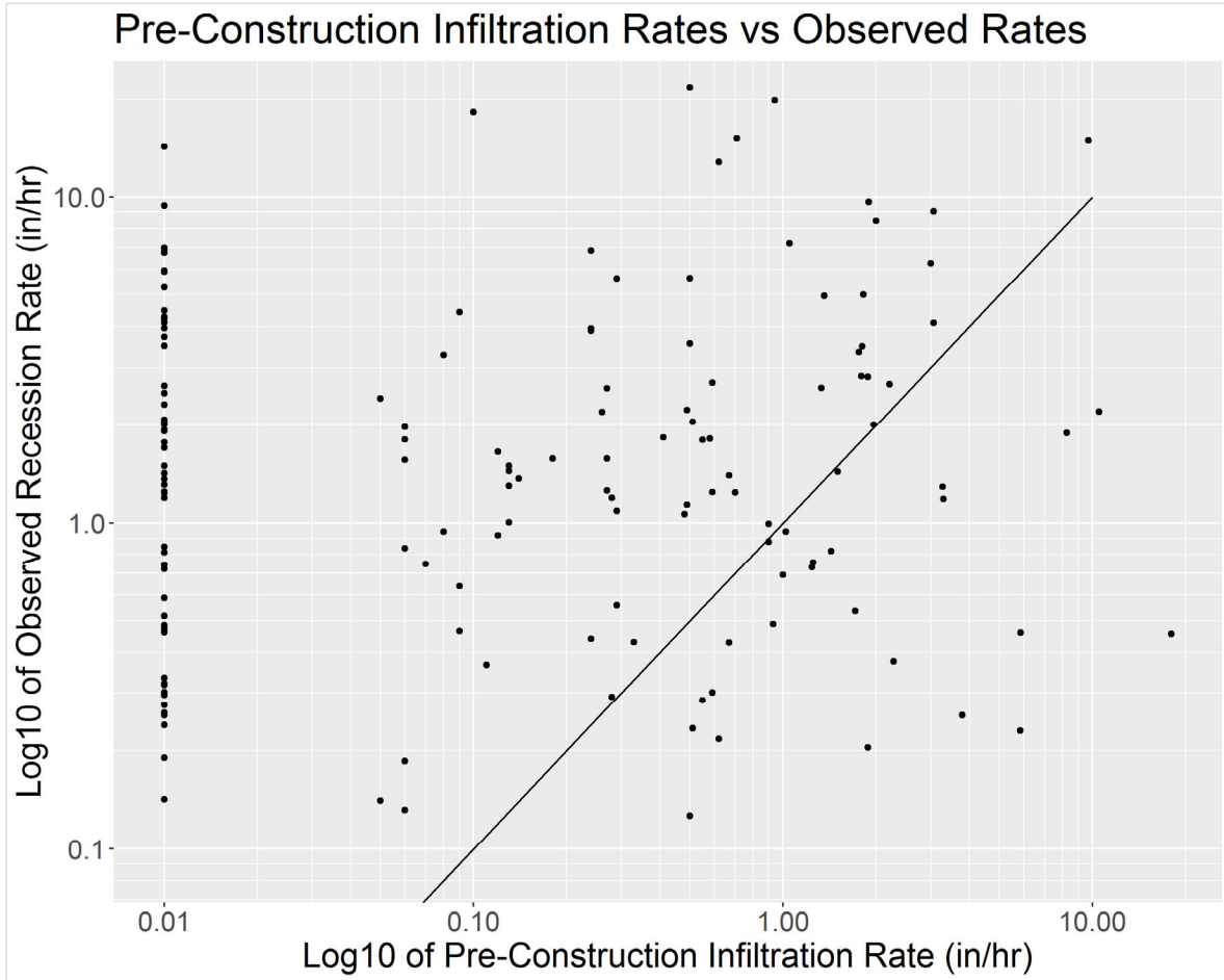
Figure 3- 4: Log-log scale scatter plot of pre-construction infiltration rates and measured saturated infiltration rates from GSI monitoring
