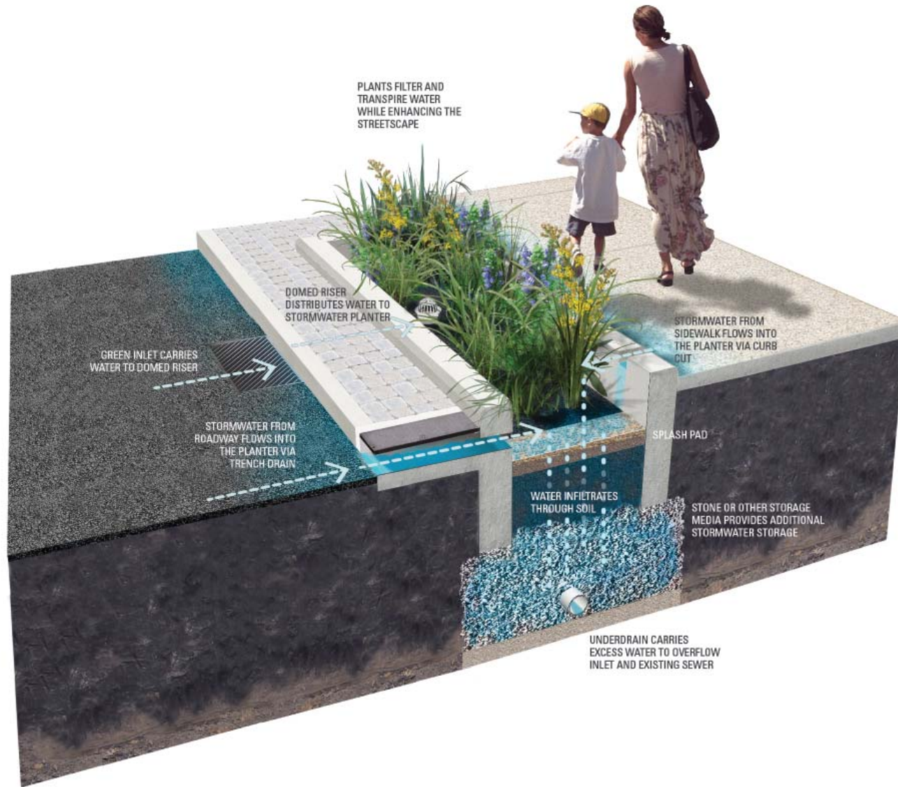
Figure 1-10. Stormwater Planter with Typical Features
