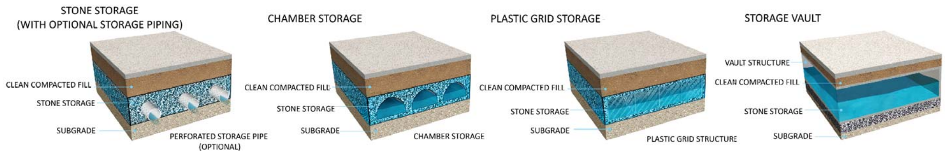
Figure 1-14. Infiltration/Storage Trench with Typical Features
