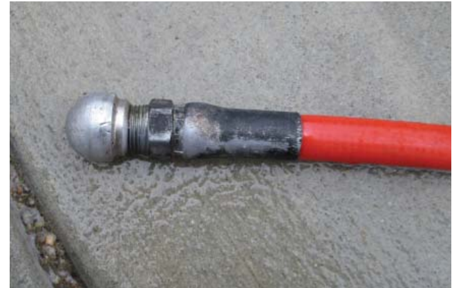
Figure 3-7. Small Penetrating Nozzle with 1 Front-facing and 6 Rear-facing Jets
