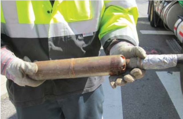
Figure 3-4. Large Penetrating Nozzle with 1 Front-Facing and 5-Rear Facing Jets
