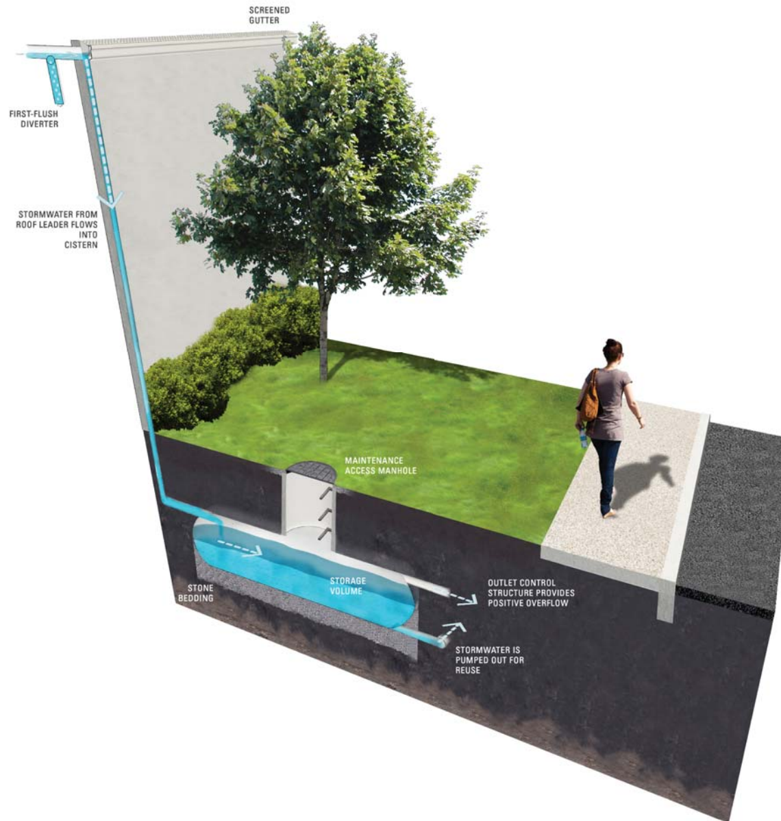
Figure 1-28. Subsurface Cistern with Typical Features
