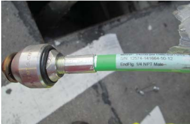
Figure 3-6: Small Rotating, Root Cutting Nozzle
