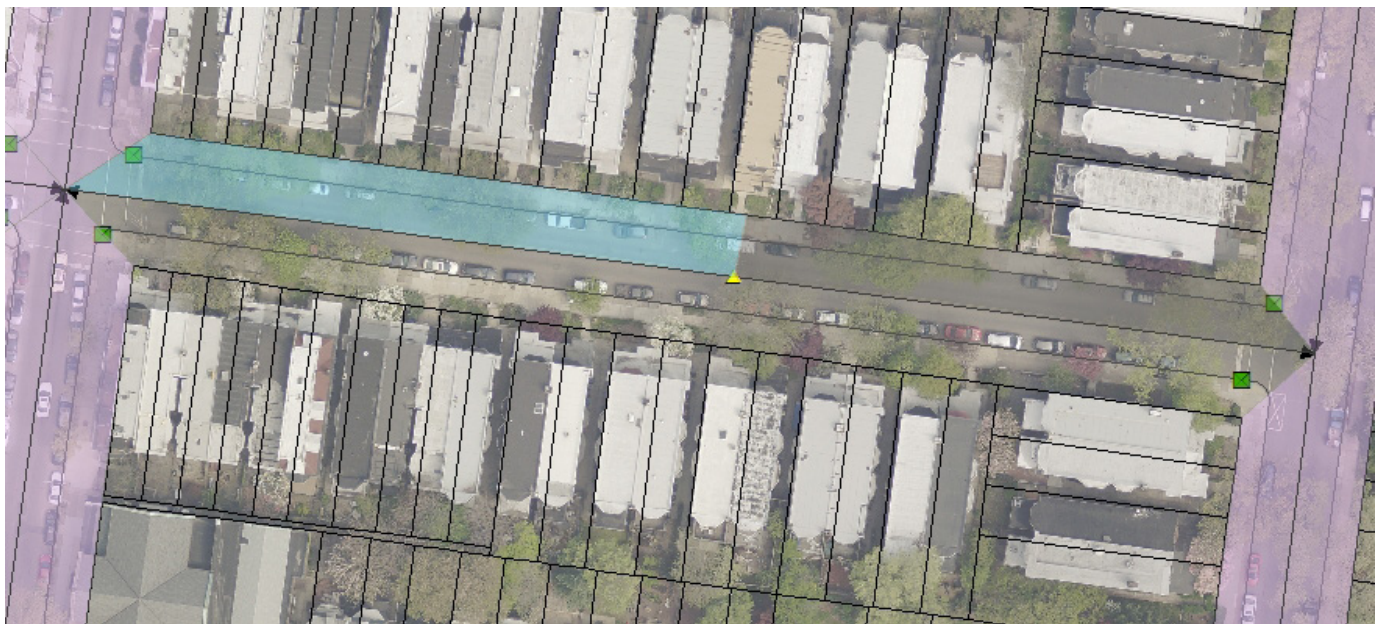
Figure 16: This image shows an example of a city block with a high point, thus splitting the typical drainage area.
