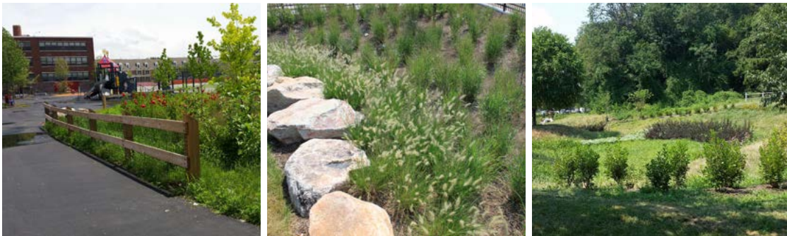
Figure 27: Images showing protection features that work well with adjacent vehicular and/or pedestrian circulation. From left to right: fence, boulders, shrub border.
