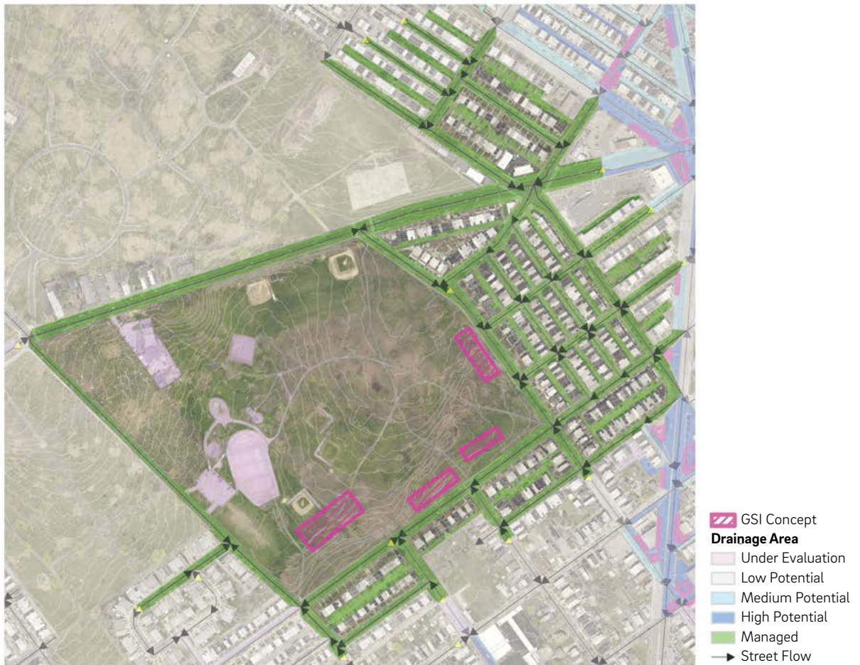
Figure 19: This example shows right-of-ways being managed by a Centralized GSI Facility on a park parcel.
