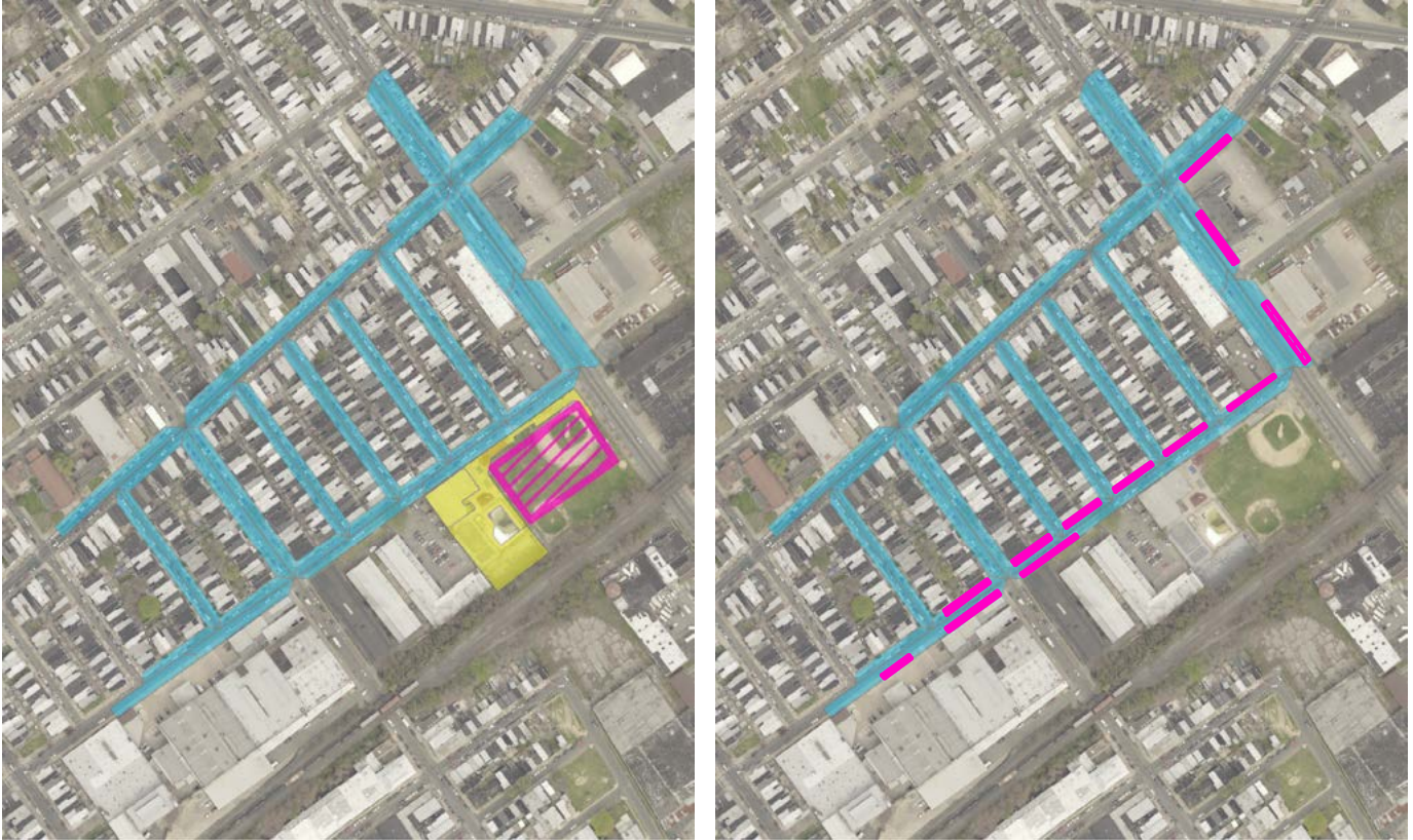
Figure 23: This example shows drainage areas that can be managed by a park (left) and by street systems (right).
