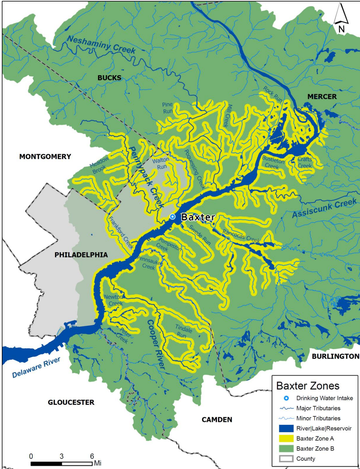
FIGURE 2-3: DELAWARE RIVER SOURCE WATER PROTECTION ZONE A RELATIVE TO THE BAXTER INTAKE (ADAPTED FROM PWD 2002A)
