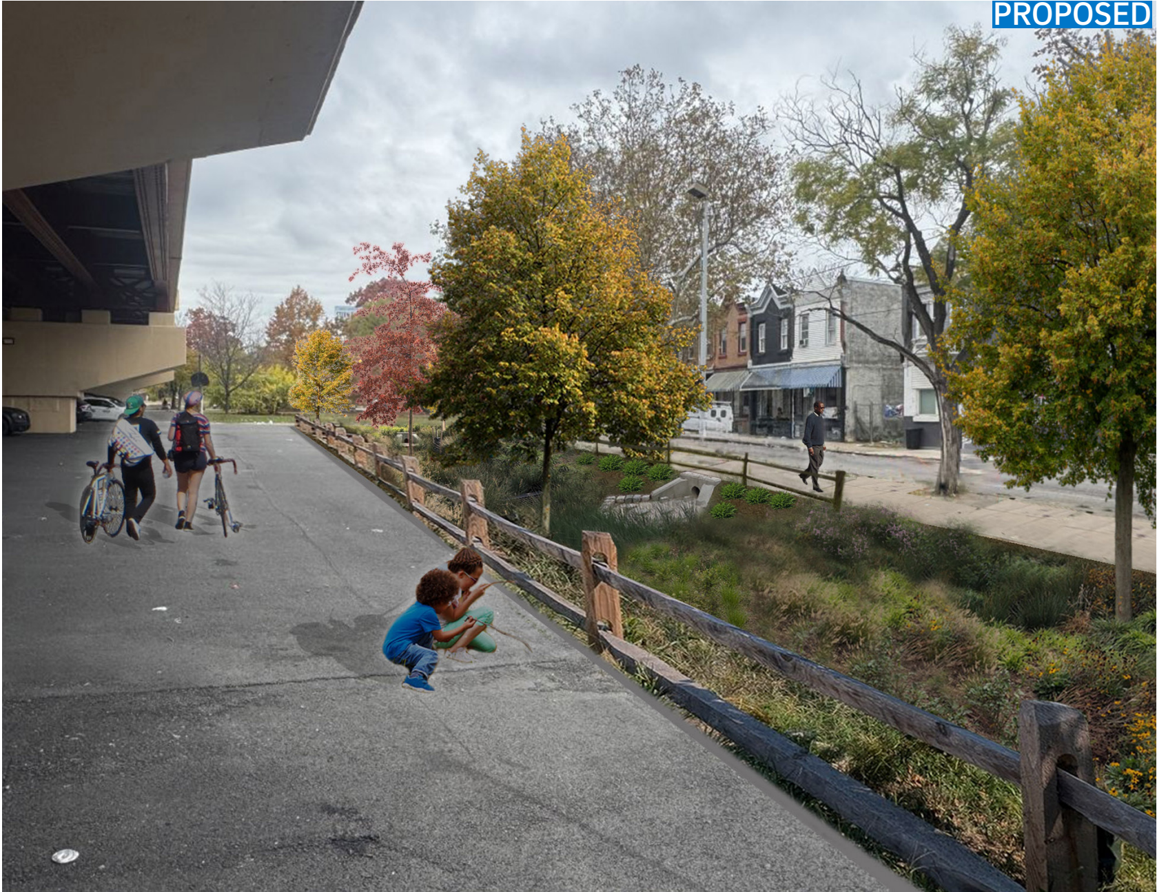
Rendering of proposed rain garden along W. Cayuga street including vegetation, split rail fencing, and stormwater infrastructure.
