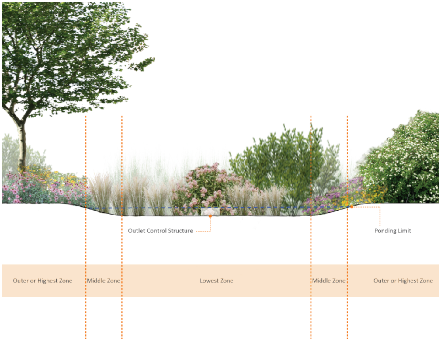
Figure 4.1-3: Hydrologic Zones of a Bioinfiltration/Bioretention Basin
