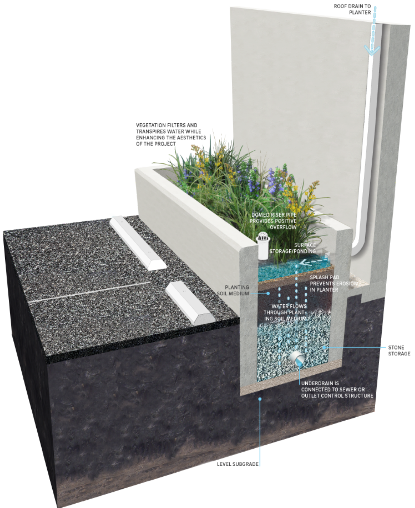
Figure 4.1-2: Flow-Through Planter Box with Typical Features
