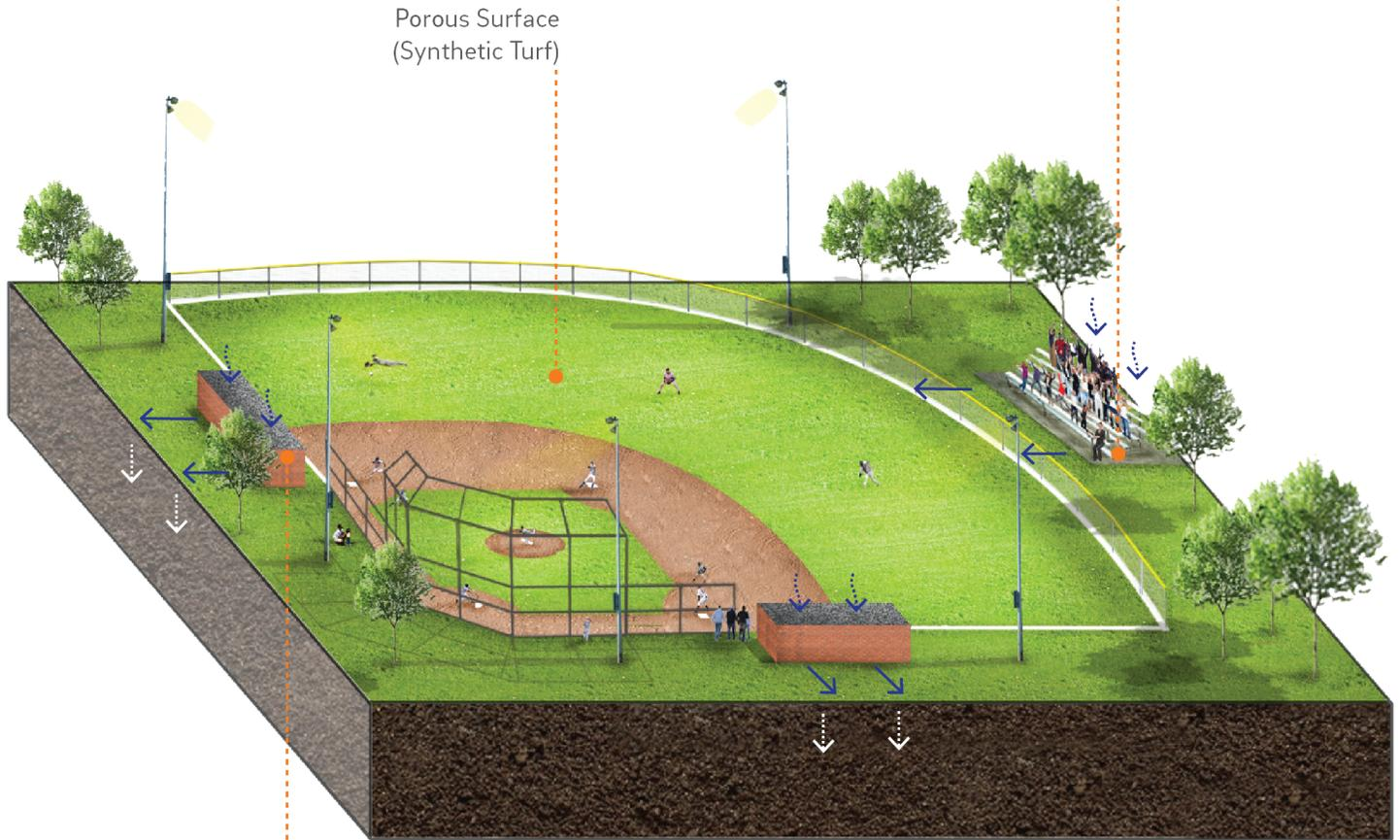
Make flow path equal to or greater in length than the dugout rooftop and make slope of pervious area less than 5% to disconnect roof area.
