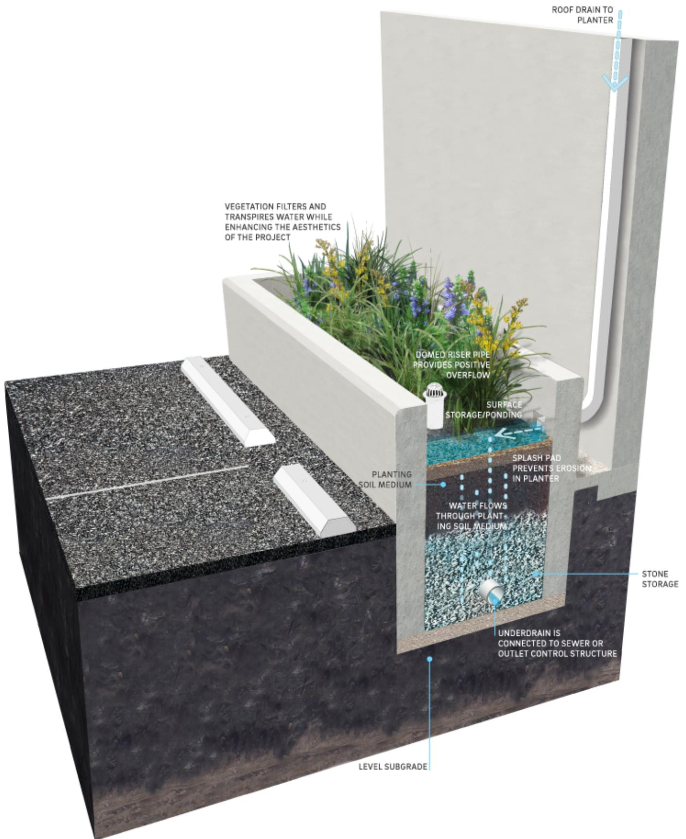
Beneath surface storage areas, prepared planting soil medium provides *subsurface storage* capacity. This storage capacity is a function of the soil depth, surface area, and void space. The planting soil medium serves as the primary Water Quality treatment mechanism of a bioinfiltration/bioretention SMP, filtering runoff before it reaches the native soil (for bioinfiltration SMPs) or before it reaches the downstream discharge point (for bioretention SMPs).
