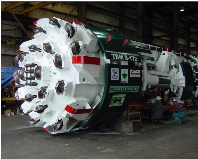
Figure 3. A TBM is a large machine designed to bore circular tunnels through hard rock and soil.
