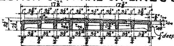
SECTION OF COVER ON LINE A-B
