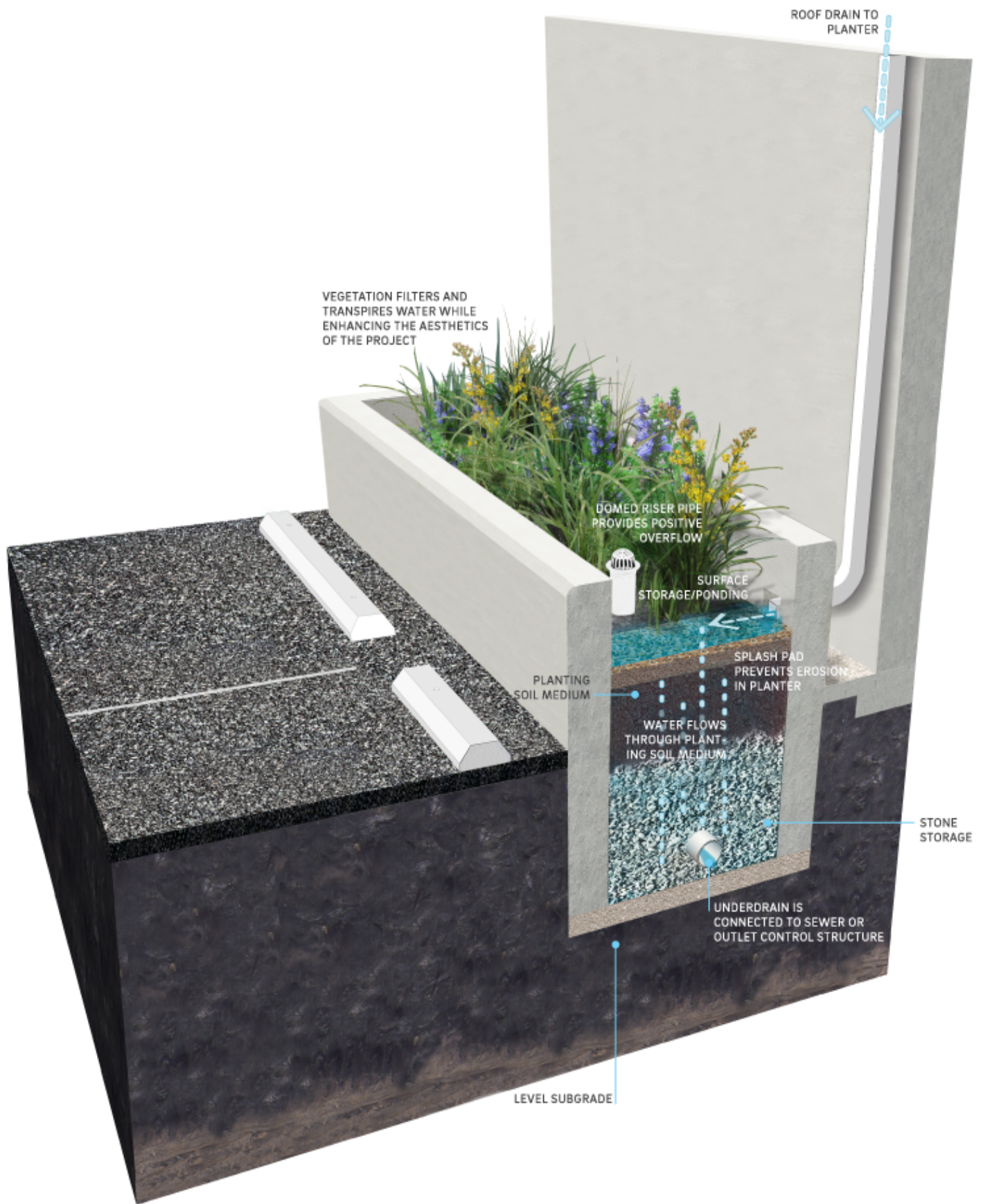
Figure 4.1-2: Flow-Through Planter Box with Typical Features
