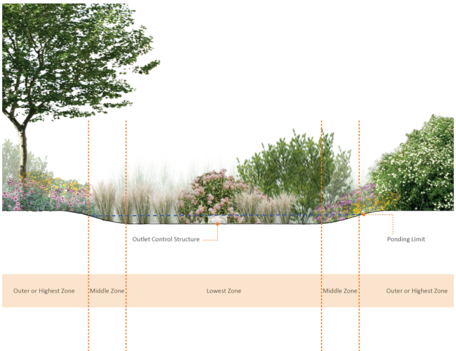
Figure 4.1-3: Hydrologic Zones of a Bioinfiltration/Bioretention Basin
