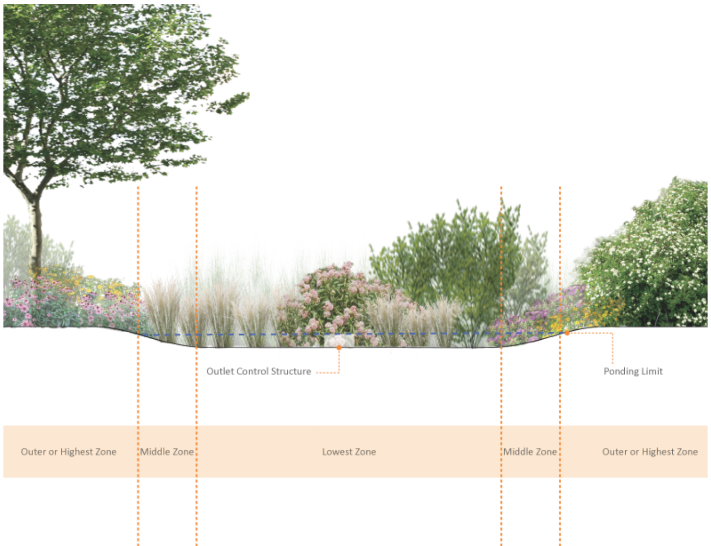
Figure 4.13-3: Hydrologic Zones of a Bioinfiltration/Bioretention Basin
