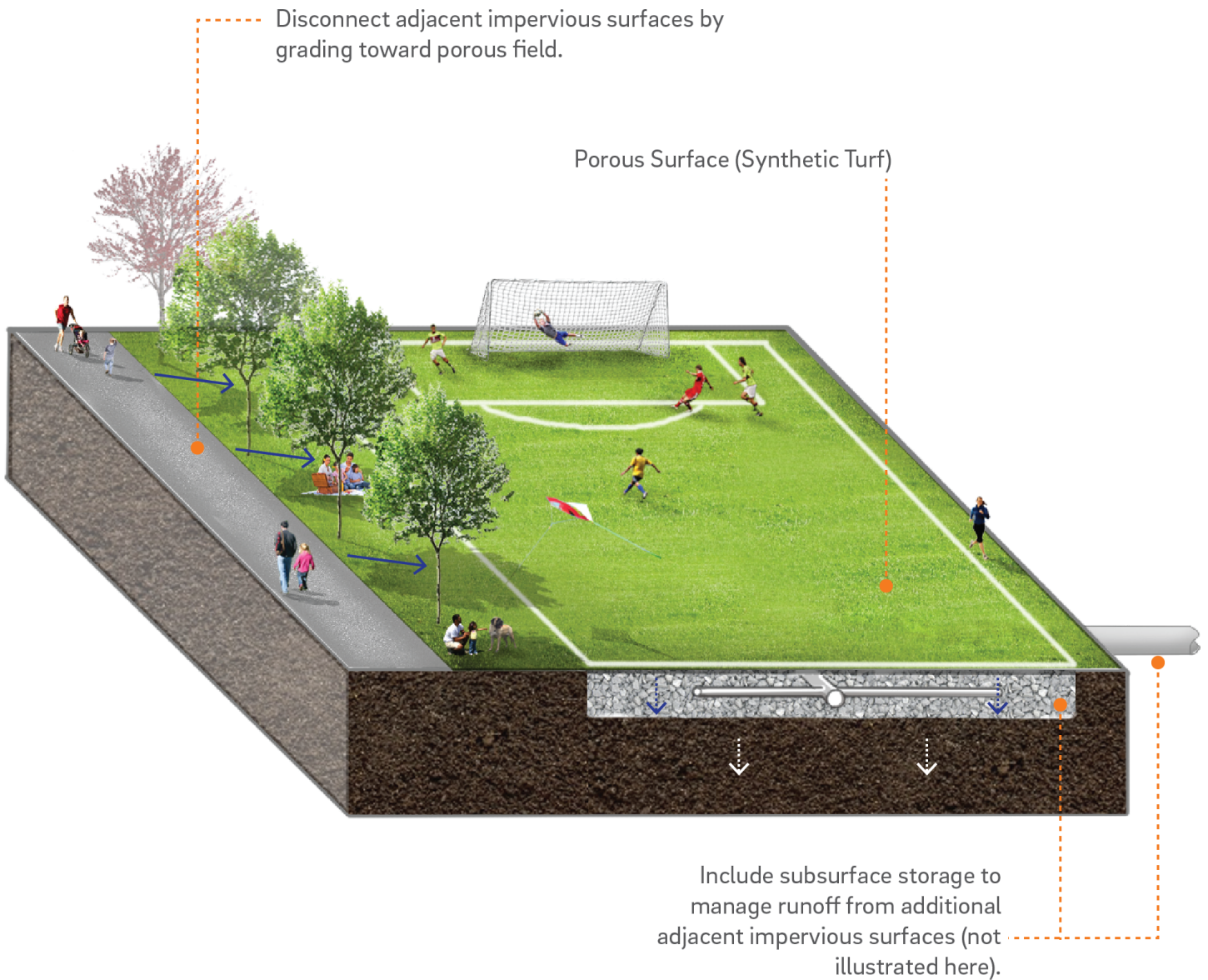
Figure 3.5-11: Athletic Field Example, Subsurface SMP to Manage DCIA
