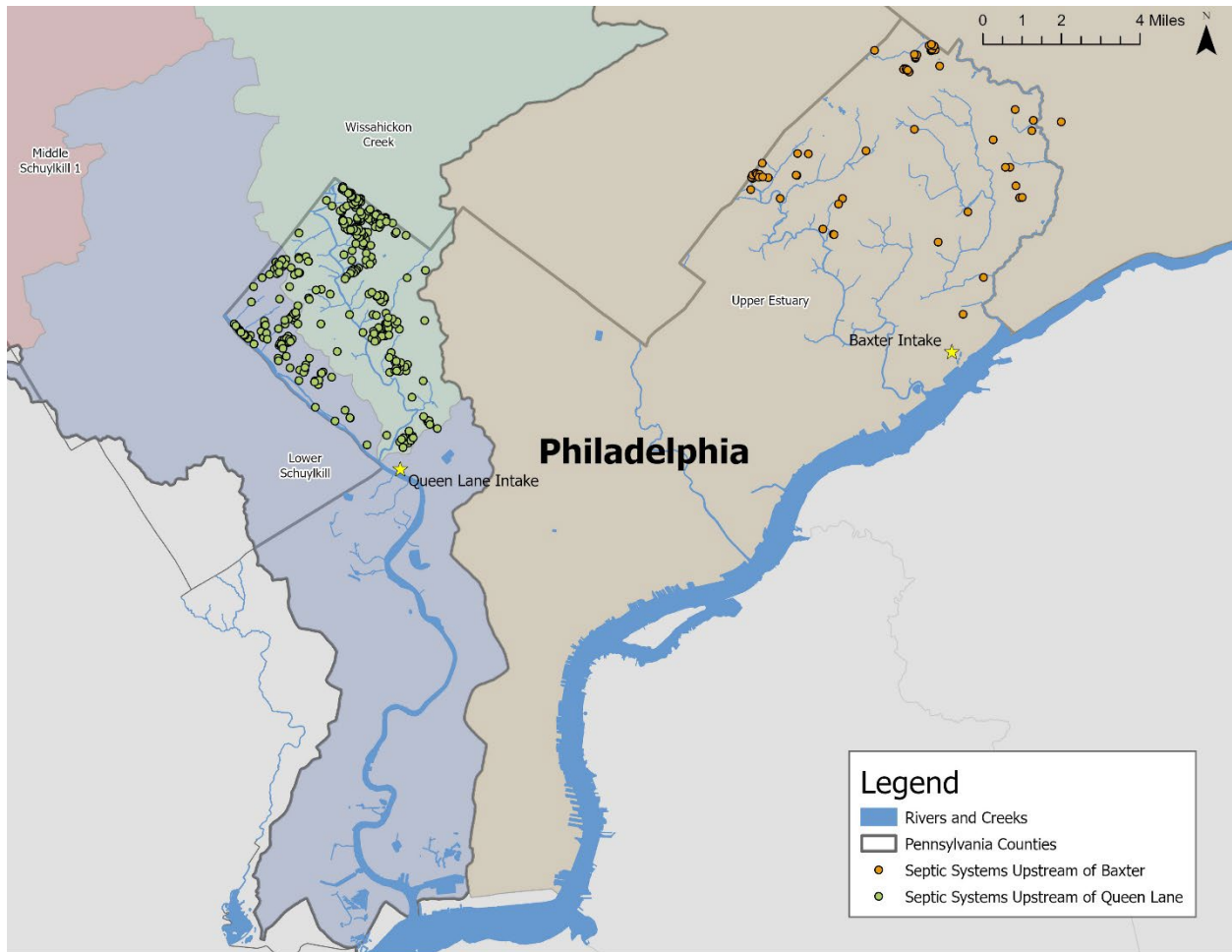
Figure 7 Map of Septic Systems in Philadelphia County Upstream of Queen Lane Water Treatment Plant
